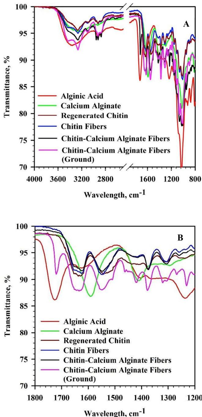
Fig.3 Full (A) and expanded (B) FT-IR spectra of commercial alginate (red), commercial calcium alginate (green), regenerated chitin powder (dark red), chitin fibers (blue), whole chitin-calcium alginate fibers (black), and ground chitin-calcium alginate fibers (pink).
