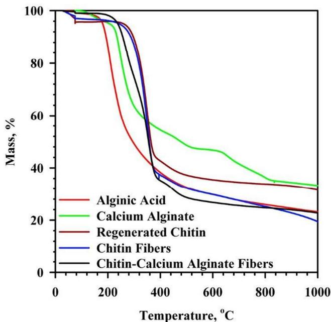
Fig.4 Comparison of TGA data for commercial alginic acid (red), commercial calcium alginate (green), regenerated chitin powder (dark red), chitin fibers (blue) and chitin-calcium alginate fibers (black).
