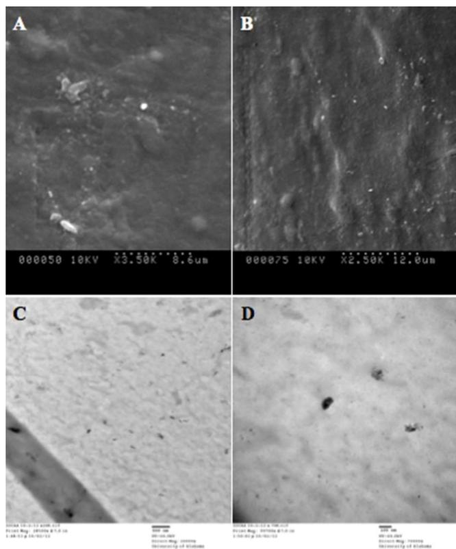
Fig.2 Selected SEM (A, B) and TEM (C, D) micrographs of chitin-calcium alginate fibers: A: 10 kV, x3.5K, 8.6  $\mu\text{m}$ ; B: 10 kV, x2.5K, 12.0  $\mu\text{m}$ ; C: 500 nm, HV 60.0 kV, Direct Mag: x20000; D: 100 nm, HV 60.0 kV, Direct Mag: x70000.
