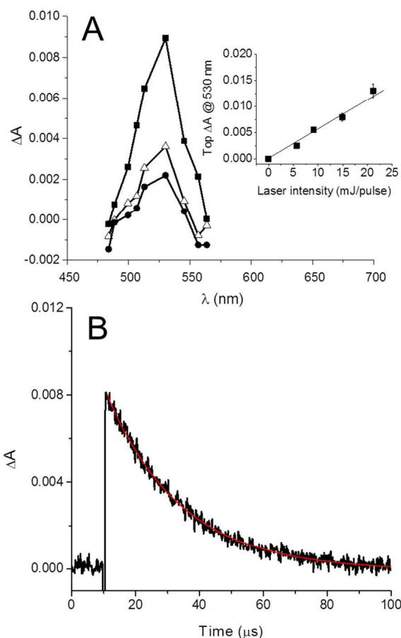
**Fig. 5** (A) Transient absorption spectra observed (■) 1  $\mu s$ , ( $\Delta$ ) 15  $\mu s$  and (●) 30  $\mu s$  after 532 nm laser excitation ( $E_{532} \sim 10$  mJ/pulse, pulse with ca. 6 ns) of the supramolecular hydrogel in air-equilibrated conditions. The inset shows the laser intensity dependence of the  $\Delta A$  monitored at 530 nm and taken 0.1  $\mu s$  after the laser pulse. (B) Decay trace monitored at 530 nm and the related first-order fitting.
