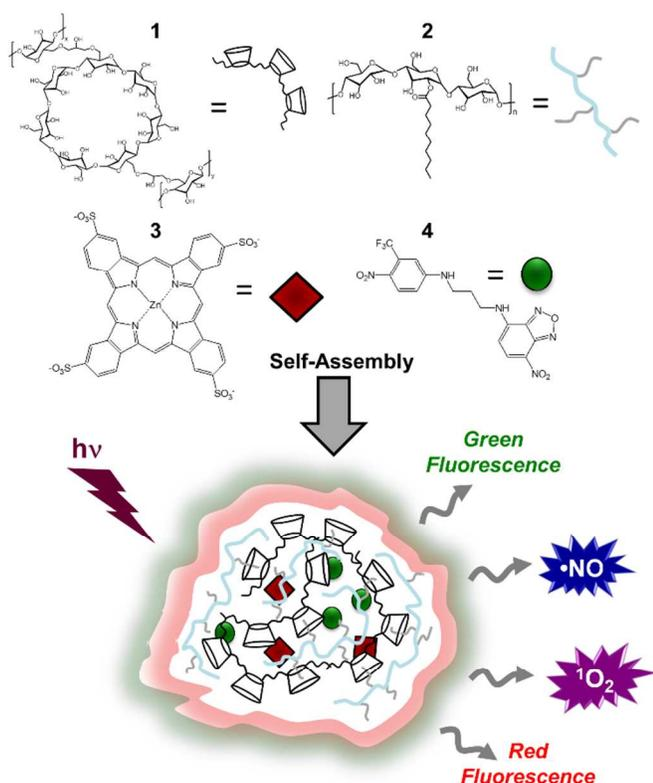
**Scheme 1.** Schematic representation of the multi-photoresponsive supramolecular hydrogel and molecular structures of the compounds used in this work.
