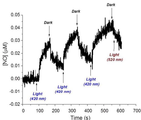
**Fig. 4** NO release profile observed upon alternate period of irradiation of the supramolecular hydrogel at 25°C.
