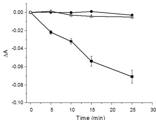
**Fig. 6** Bleaching of the RNO absorption at 440 nm as a function of the time observed in the presence of the hydrogel in the dark ( $\Delta$ ) and upon irradiation with  $\lambda_{\text{exc}} = 680$  nm ( $\blacksquare$ ), and in the absence of the hydrogel ( $\bullet$ ) upon irradiation with  $\lambda_{\text{exc}} = 680$  nm. [RNO] = 47  $\mu\text{M}$ ; [imidazole] = 10 mM. Cell pathlength = 1 cm. Phosphate buffer 10 mM, pH 7.4, 25°C.
