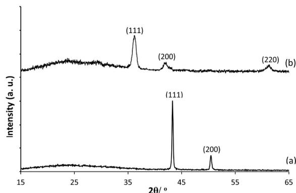
Figure 1. Powder XRD pattern for (a) a Cu film deposited from [Cu(NO<sub>3</sub>)<sub>2</sub>·3H<sub>2</sub>O] in methanol at 350 °C and cooling under N<sub>2</sub> and (b) a Cu<sub>2</sub>O film deposited from [Cu(NO<sub>3</sub>)<sub>2</sub>·3H<sub>2</sub>O] in methanol at 350 °C and cooling in air.
