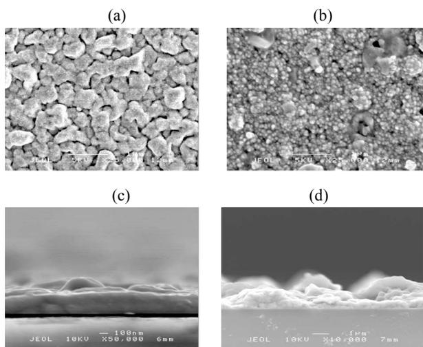
Figure 2. SEM micrograph of (a) Cu film grown via AACVD of  $[\text{Cu}(\text{NO}_3)_2 \cdot 3\text{H}_2\text{O}]$  in methanol at 350  $^{\circ}\text{C}$  and cooled under  $\text{N}_2$  and (b) a  $\text{Cu}_2\text{O}$  film deposited from  $[\text{Cu}(\text{NO}_3)_2 \cdot 3\text{H}_2\text{O}]$  in methanol at 350  $^{\circ}\text{C}$  and cooled in air. Side-on SEM of (c) the Cu film and (d) the  $\text{Cu}_2\text{O}$  film.
