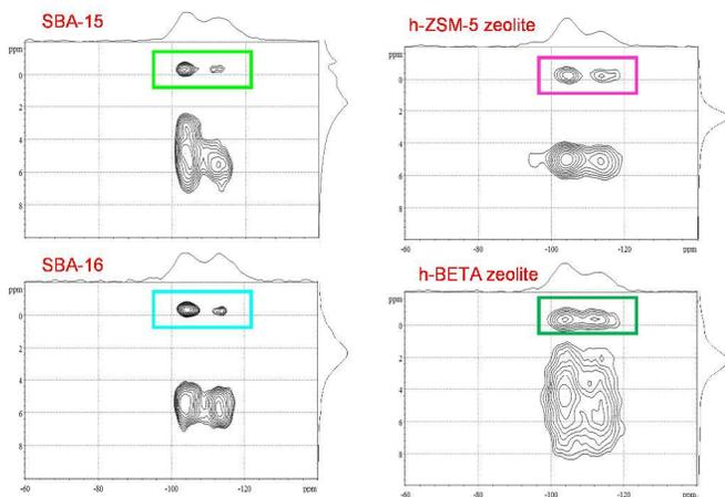
Figure 4. Solid-state  $^1\text{H}$ - $^{29}\text{Si}$  HETCOR NMR spectra of methylprednisolone hemisuccinate confined in mesoporous and hierarchical zeolitic materials and the corresponding  $^1\text{H}$  and  $^{29}\text{Si}$  projections
