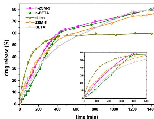
Figure 3. Methylprednisolone hemisuccinate release percentages as a function of release time by using the hierarchical zeolites as carriers
