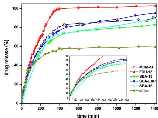
Figure 2. Methylprednisolone hemisuccinate release percentages as a function of release time by using the ordered mesoporous silica materials as carriers
