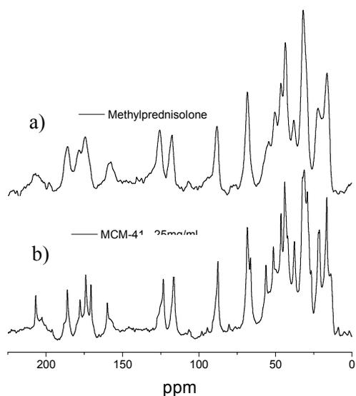
Figure 1. Solid-state  $^{13}\text{C}$  NMR spectrum of (a) pure methylprednisolone hemisuccinate and (b) methylprednisolone hemisuccinate load onto mesoporous MCM-41 material
