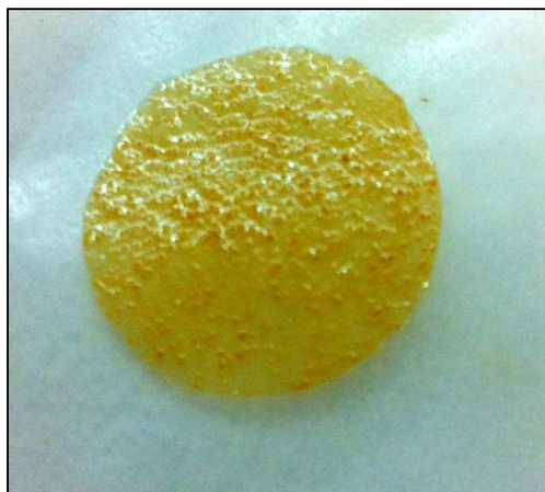
Figure 5. The PVDF-HFP/MTF-Li electrolyte membrane.
