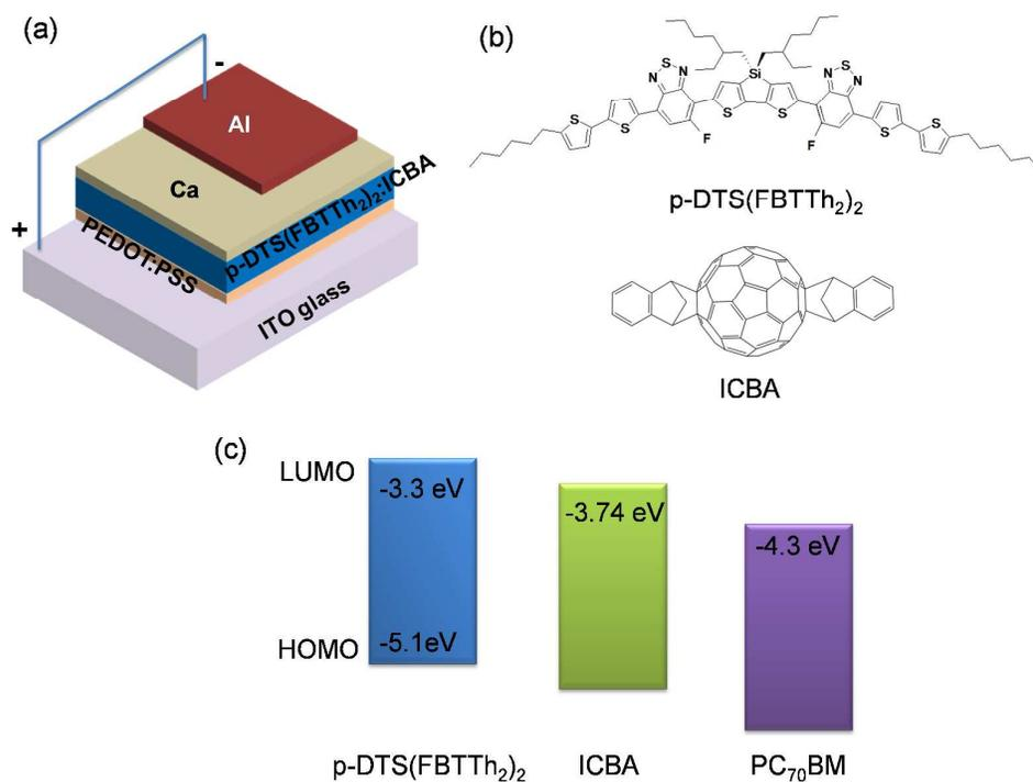
**Fig. 1** Device structure of organic solar cell with p-DTS(FBTTh<sub>2</sub>)<sub>2</sub>:ICBA blend used in this study (a). Molecular structure (b) and energy level (c) of p-DTS(FBTTh<sub>2</sub>)<sub>2</sub> and ICBA, respectively. LUMO level of PC<sub>70</sub>BM is shown in (c) for comparison with ICBA.
