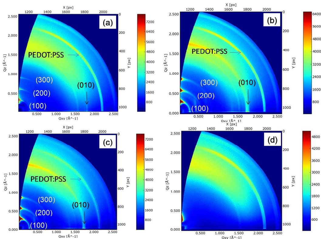
**Fig. 4** 2D GIWAXS patterns of p-DTS(FBTTh<sub>2</sub>)<sub>2</sub>:ICBA films fabricated on PEDOT:PSS coated substrate using different processing conditions: as cast (a), 0.4% DIO and annealed at 120 °C (b), 0% DIO and annealed at 100 °C (c). The 2D GIWAXS patterns of PEDOT:PSS film is shown in (d).
