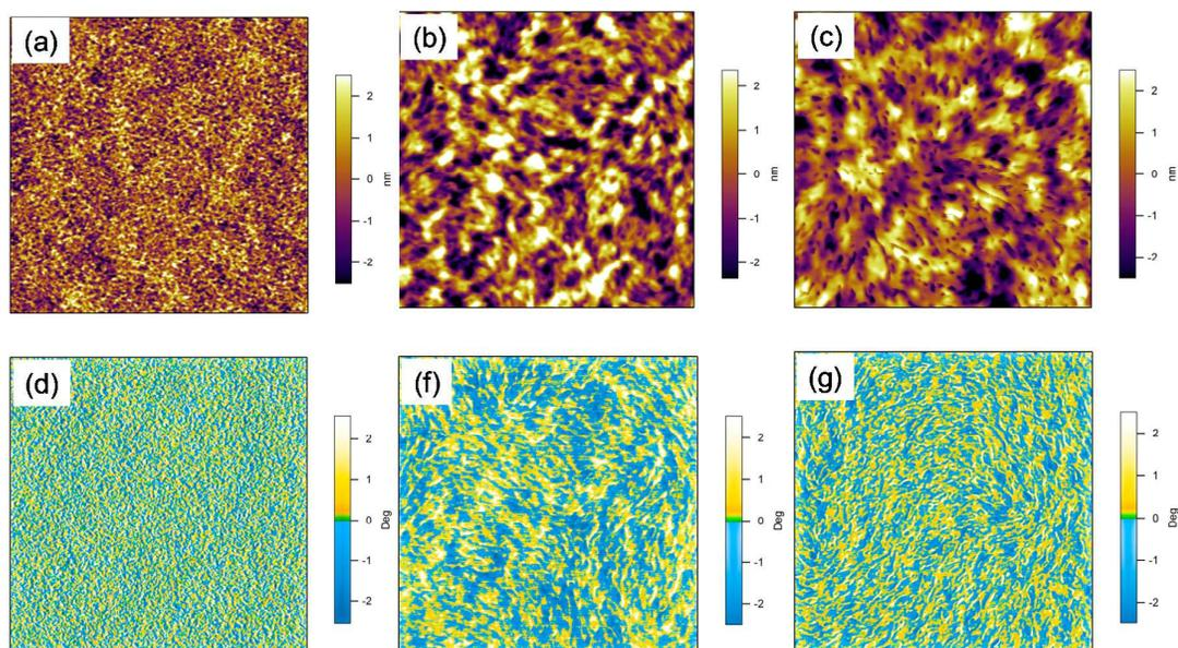
**Fig. 3** Tapping mode AFM topography (top) and phase (bottom) images of p-DTS(FBTTh<sub>2</sub>)<sub>2</sub>:ICBA films fabricated using different processing conditions: as cast (a & d), 0.4% DIO and annealed at 120 °C (b & f), and 0% DIO and annealed at 100 °C (c & g). D:A ratio is 1.5:1 for all films. The scan size is 2 μm × 2 μm.
