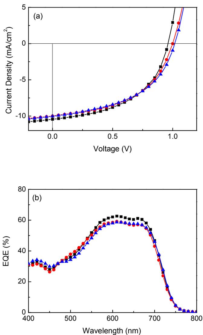
**Fig. 2** (a)  $J$ - $V$  characteristics under AM 1.5G irradiation at  $100 \text{ mW/cm}^2$  and (b) EQE spectra of the champion cells fabricated from different processing conditions: (i) D:A = 1.5:1, 0.4% DIO and annealed at  $120 \text{ }^\circ\text{C}$  (black square), (ii) D:A = 1.5:1, 0% DIO and annealed at  $100 \text{ }^\circ\text{C}$  (red circle) and (iii) D:A = 2.3:1, 0% DIO and annealed at  $100 \text{ }^\circ\text{C}$  (blue triangle).
