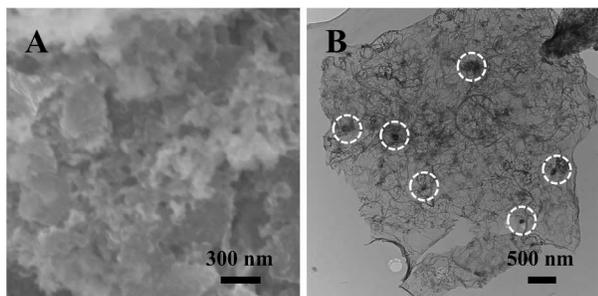
**Figure 5.** (A) SEM and (B) TEM images of the electrode after charge-discharge cycling for 100 cycles at the voltage range between 1.500 to 0.005 V vs. Li/Li<sup>+</sup>. The white dashed circles point out several places where Si NPs exist.
