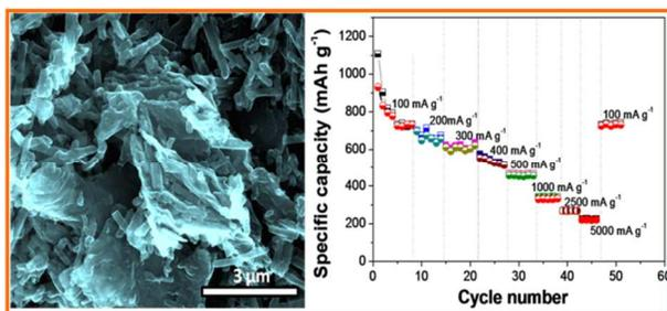
Novel approach to synthesis nitrogen rich (few layer graphene-carbon nanotube) hybrid nanomaterial for high performance Li ion battery anode electrodes.
