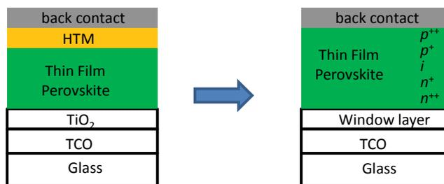
Figure 9: The proposed hole-conductor-free perovskite solar cell without HTM layer by utilizing  $p$ -type doping.
