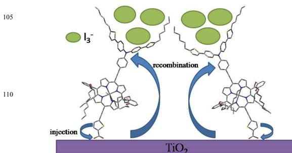
**Fig. 6** Anchoring unit affects the dye JP3's orientation on the  $TiO_2$  surface
