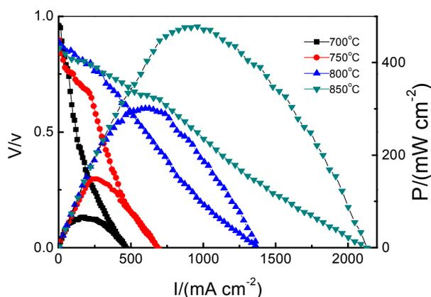
**Figure 8** Output of MT-SOFC based on the LSM-YSZ/LSM dual-layer hollow fibers ( $\text{H}_2$  feed flow rate =  $40 \text{ mL min}^{-1}$ ; air feed flow rate =  $90 \text{ mL min}^{-1}$ ).
