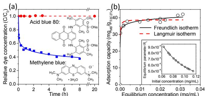
**Fig. 2.** (a) Time dependence of MB ( $C_0 = 0.05 \text{ mg}/\text{mL}$ ) and AB 80 ( $C_0 = 0.06 \text{ mg}/\text{mL}$ ) concentrations in aqueous solutions with suspended  $\text{Ti}_3\text{C}_2\text{T}_x$  particles in the dark. Chemical structures of corresponding dyes are shown as insets. (b) Adsorption isotherms of MB on  $\text{Ti}_3\text{C}_2\text{T}_x$ . Inset shows dependence of the equilibrium parameter  $R_L$  (see Eq. 2, ESI†) on initial concentration,  $C_0$ , of MB.
