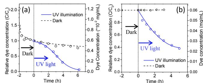
**Fig. 5.** Time dependence of relative concentrations,  $C/C_0$ , of, (a) MB and, (b) AB80 in  $\text{Ti}_3\text{C}_2\text{T}_x$  containing solutions. Solid and dashed lines correspond to measurements taken under UV light and in the dark, respectively.
