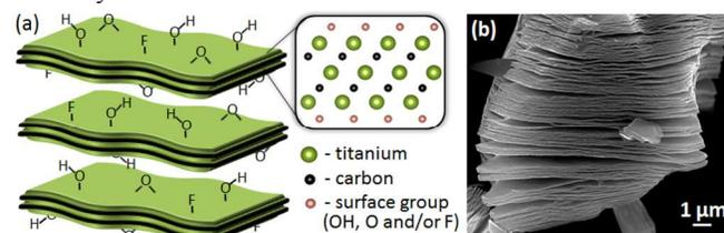
**Fig. 1.** (a) Schematic of  $\text{Ti}_3\text{C}_2\text{T}_x$  layered structure with a side view atomic model of a single sheet. (b) SEM image of a  $\text{Ti}_3\text{C}_2\text{T}_x$  particle.
