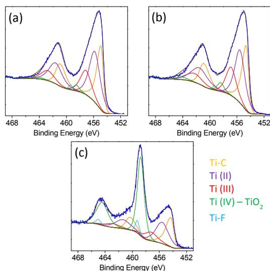
**Fig. 4.** High-resolution XPS in the Ti 2p region for  $\text{Ti}_3\text{C}_2\text{T}_x$ , (a) before MB adsorption, (b) after 20 h MB adsorption, (c) after 1 week in a 0.05 mg/mL MB aqueous solution shaken in the dark in aerated conditions. The fits are color-coded; the key is shown on the right of (c). An increase in the Ti  $2p_{3/2}$  component corresponding to  $\text{TiO}_2$  (colored green) can be observed at 458.8 eV.
