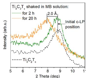
**Fig. 3.** X-Ray diffraction patterns around the  $\text{Ti}_3\text{C}_2\text{T}_x$  (0002) peak after soaking in aqueous  $0.05 \text{ mg}/\text{mL}$  MB solution for 2 h and 20 h.
