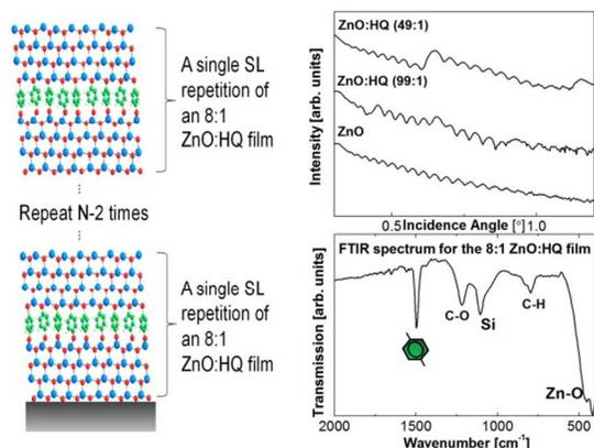
Figure 1. The layered SL structure of the (Zn,Al)O:HQ thin films; the XRR and FTIR data are for the ZnO:HQ compositions of 99:1, 49:1 and 8:1 (made for FTIR only), respectively.
