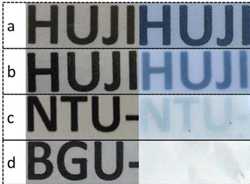
Figure 4 Smart hydrogel thin films at room temperature (left) and in sunshine environment at 35 °C (right) with thickness of (a) 26  $\mu\text{m}$ ; (b) 52  $\mu\text{m}$ ; (c) 78  $\mu\text{m}$  and (d) 200  $\mu\text{m}$ .
