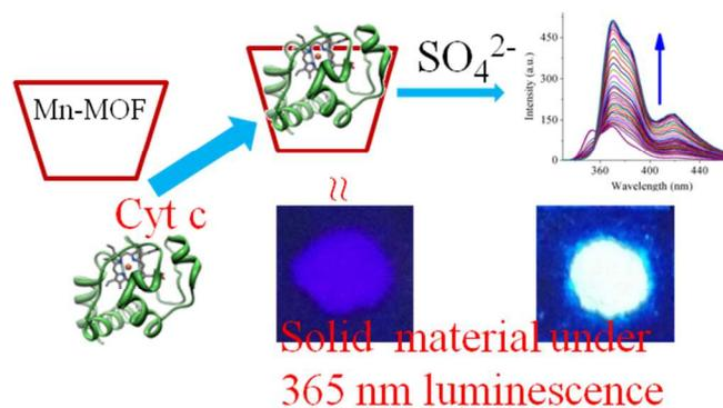
An ensemble of cytochrome c and 2, 6 naphthalene dicarboxylate based metal organic framework is synthesized. The bio-material selectively sense sulfate ions in 100 % aqueous solution.
