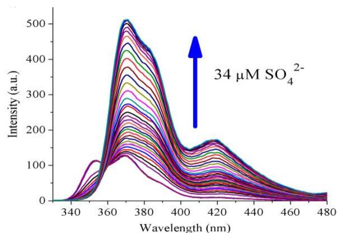
**Figure 3:** Fluorescence emission spectrum of **5** on addition of  $34 \mu\text{M}$  of  $\text{SO}_4^{2-}$  ions.
