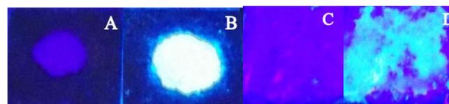
**Figure 6:** Solid state luminescence photographs of (A) **5** (B) **5** +  $\text{SO}_4^{2-}$  (C)  $\text{SO}_4^{2-}$  adsorbed on clay (D) after addition of **5** to  $\text{SO}_4^{2-}$  adsorbed on clay under luminescence (UV) emission of 365 nm.
