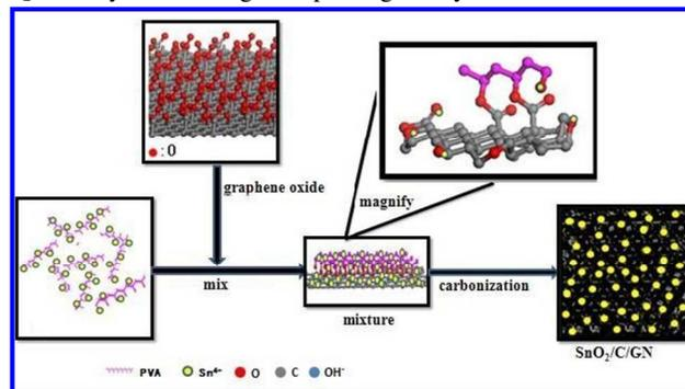
**Fig. 5** Synthesis schematic and the structure of SnO<sub>2</sub>/C/GN voids existing between individual composite sheets could be fixed by carbonized PVA for stabilization. Graphene oxide sheets act as crystal nucleuses for promoting the growth and distribution of SnO<sub>2</sub> nanocrystals, which have been approved by XRD and TEM.
