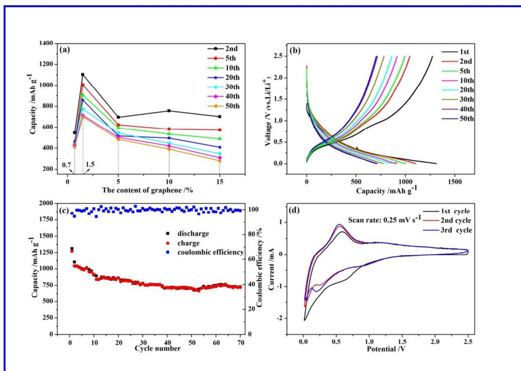
**Fig. 7** (a) Specific capacity vs. graphene content, (b) the charge/discharge profiles of SnO<sub>2</sub>/C/GN-1.5, (c) the cyclic performance of SnO<sub>2</sub>/C/GN-1.5 and (d) the cyclic voltammograms of SnO<sub>2</sub>/C/GN-1.5
