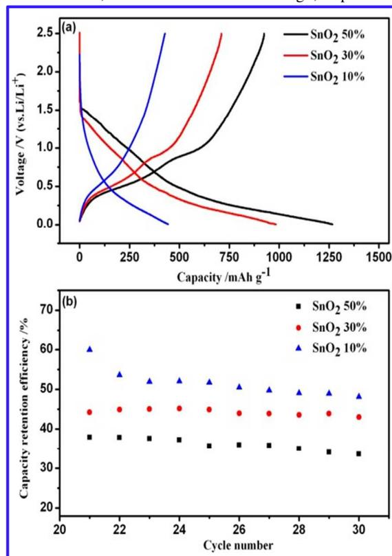
**Fig. 6** (a) Charge/discharge profiles and (b) capacity retention efficiency profiles of SnO<sub>2</sub>/C-10, SnO<sub>2</sub>/C-30 and SnO<sub>2</sub>/C-50
