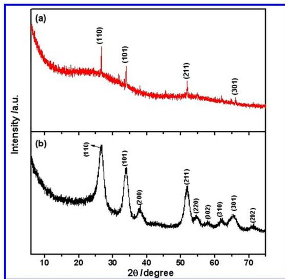
**Fig. 1** XRD patterns of (a) SnO<sub>2</sub>/C/GN-1.5 and (b) SnO<sub>2</sub>/GN
