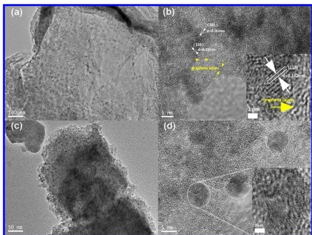
**Fig. 4** TEM images of (a) SnO<sub>2</sub>/C/GN-1.5, (c) SnO<sub>2</sub>/C-50 and HRTEM images of (b) SnO<sub>2</sub>/C/GN-1.5, (d) SnO<sub>2</sub>/C-50
