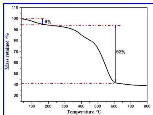
**Fig. 3** TGA curve of SnO<sub>2</sub>/C/GN-1.5 in air and 0.26 nm respectively corresponding to (110) and (101) planes of SnO<sub>2</sub>. Thin layers of carbon in form of stacked graphene sheets can be found on the edges of SnO<sub>2</sub> particles (*cf.* arrows). Therefore, the
