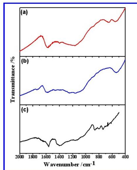
**Fig. 2** FT-IR spectra of (a) SnO<sub>2</sub>/C/GN-1.5, (b) SnO<sub>2</sub>/C-50 and (c) C-PVA
