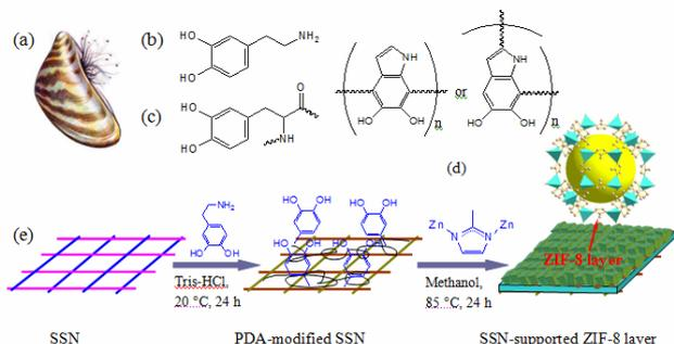
**Fig. 1.** Mussel with byssus threads (a), chemical structure of DPA (b), DOPA (c), and PDA (d), schema of the preparation of ZIF-8 molecular sieve membrane on PDA-functionalized SSN (e).
