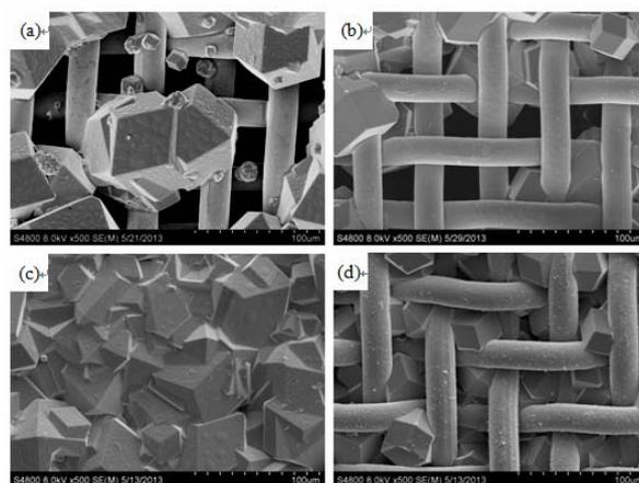
**Fig. 2.** FESEM images of upper side (a) and down side (b) of the ZIF-8 layer prepared for 24 h on non-modified SSN, FESEM images of upper side (c) and down side (d) of the of ZIF-8 membrane prepared for 24 h on PDA-functionalized SSN. The attributes “upper” and “down” refer to the horizontal orientation of the SSN in ZIF-8 membrane synthesis.
