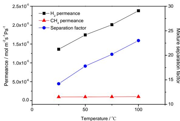
**Fig. 6.** Gas permeances and  $H_2/CH_4$  selectivity of the ZIF-8 membrane supported on PDA-functionalized SSN as a function of the temperature at 1 bar.
