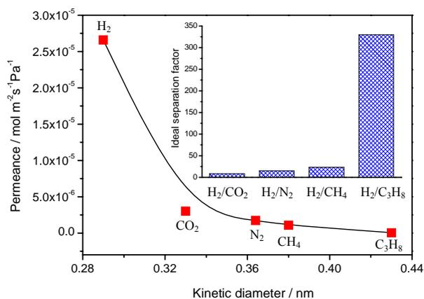
**Fig. 5.** Single gas permeances on the ZIF-8 membrane prepared on PDA-functionalized SSN at 100 °C and 1 bar as a function of the kinetic diameter. The inset shows the mixture separation factors for  $H_2$  over other gases from equimolar mixtures as determined by gas chromatography.
