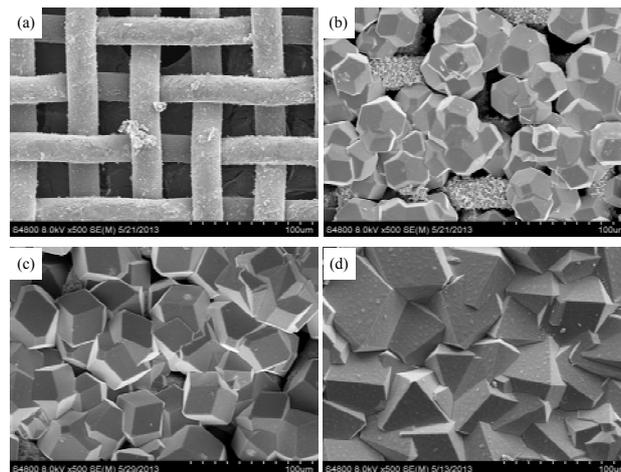
**Fig. 4.** FESEM images of ZIF-8 layer prepared on DPA-functionalized SSN with different synthesis time: 4 h (a), 8 h (b), 16 h (c), and 24 h (d).
