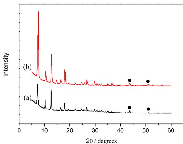
**Fig. 3.** XRD patterns of the ZIF-8 layer prepared on non-modified SSN (a), and PDA-functionalized SSN. (●): SSN, (not marked): ZIF-8 crystals.
