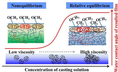
Surface structure of poly(methyl methacrylate) films influenced by chain entanglement in the corresponding film-formation solution
