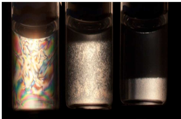
Figure 14 Mixed beidellite/silica suspensions observed between crossed polarisers one month after preparation. Volume fraction clay = 0.41% , silica = 0, 0.034, 0.138 % from left to right. Reproduced with permission from Landman et al. 148 Copyright 2014 American Chemical Society.
