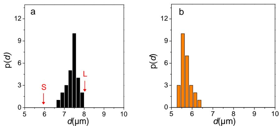
**Fig. 4** Comparison of  $p(d)$  of a PAS for  $L = 8.0 \mu\text{m}$ ,  $S = 5.9 \mu\text{m}$ ,  $a = 7.2 \mu\text{m}$  shown in a) (see also Fig. 2(c)), and a conventional two-dimensional colloidal crystal b), the later formed at smaller mean particle distance  $a = 6.0 \mu\text{m}$  in the absence of a quasiperiodic substrate potential. Both structures are formed at  $V_0 = 1.5 k_B T$ .
