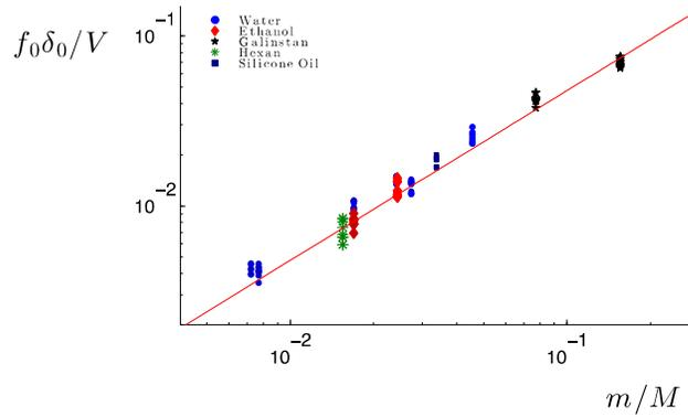
Figure 5. Normalized deflection  $f_0 \delta_0 / V$  as a function of the ratio  $m/M$  between drop and plate mass.  $V$  varies from 20 cm/s to 6 m/s. The red line shows equation  $y = (3/2\pi) x$ , that is, Eq. 2. Each color corresponds to a liquid, and each cluster to different radii  $R$  between 0.9 and 1.7 mm.
