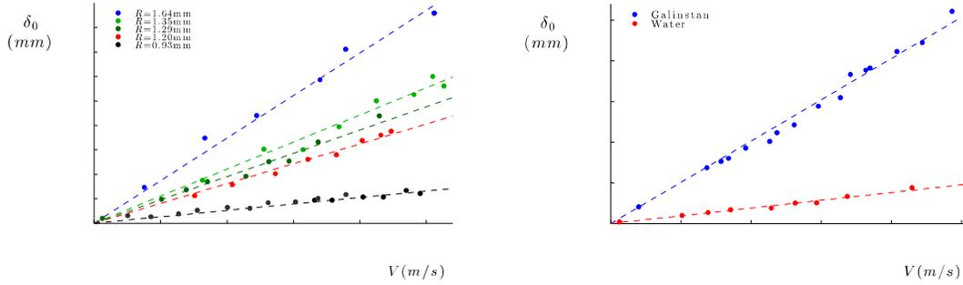
Figure 4. (a) Maximal deflection  $\delta_0$  of the tip of a glass lamella as a function of the impacting speed of a water drop hitting this lamella close to the edge. We do not observe a parabolic relationship between  $\delta_0$  and  $V$ , but a linear law. (b) Comparison between water (lower curve) and Galinstan (upper curve) for a radius  $R = 1.3$  mm. The ratio of  $\delta_0$  between the liquids is approximately the ratio of their densities.
