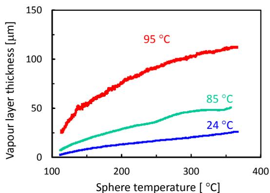
**Figure 8.** Vapour layer thickness vs sphere temperature for 20 mm superhydrophobic steel sphere cooling in 24 °C water (blue line), 85 °C (green line) and 95 °C water (red line), calculated using Fig. 2b data and eq. 4.
