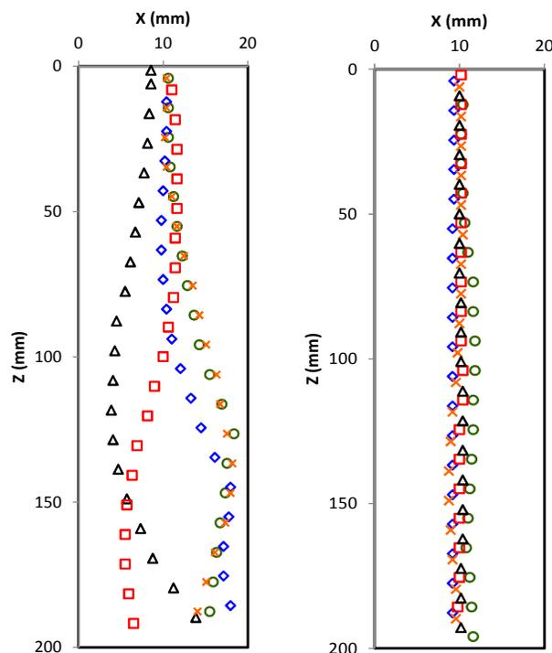
**Figure 7.** Examples of the trajectories of  $40$  mm steel falling spheres in  $95$  °C water: (a)  $T_s = 95$  °C hydrophilic spheres with no vapour layer, (b)  $T_s = 200$  °C superhydrophobic spheres in the Leidenfrost regime in the presence of a vapour layer. The horizontal and vertical ( $X, Z$ ) trajectory coordinates are obtained from high speed video recording of five independent runs with each trajectory represented by a different symbol.
