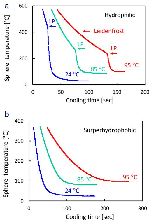
**Figure 2.** Sphere temperature vs cooling time for statically held 20 mm steel sphere cooling in 24 °C water (blue line), 85 °C (green line) or 95 °C water (red line): (a) hydrophilic sphere, (b) superhydrophobic sphere. Arrows on (a) mark the Leidenfrost point (LP) characterized by an explosive transition to the nucleated boiling regime.<sup>3</sup> Supplementary Fig. S2 shows data for the corresponding heat transfer coefficients.
