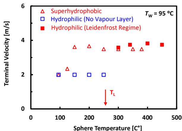
**Figure 4.** Variation of the terminal velocity with the sphere temperature, measured for a 20 mm steel sphere falling through 95 °C water. Open squares (blue) are data for hydrophilic spheres at temperature below the Leidenfrost temperature ( $T_L = 260$  °C) and solid squares (red) for temperatures above  $T_L$ . Open triangles (red) are data for superhydrophobic spheres (see also Video 1).
