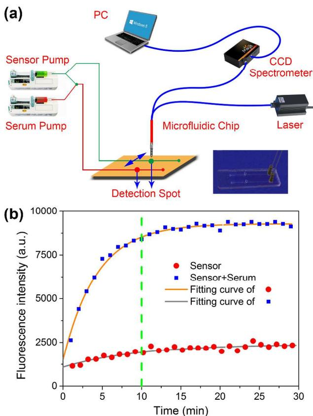
**Fig. 5** (a) Schematic diagram of microfluidic system. Inset: picture of the microfluidic chip. (b) Fluorescence response of probe **3** (10  $\mu\text{M}$ ) with/without addition of human serum acquired in a microfluidic chip.  $\lambda_{\text{ex}} = 430 \text{ nm}$ ,  $\lambda_{\text{em}} = 552 \text{ nm}$ .
