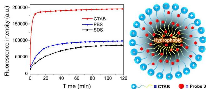
Fig. 2 (a) Fluorescence kinetics of probe **3** (10  $\mu$ M) upon addition of  $\alpha$ -KA (100  $\mu$ M) with CTAB (1 mM), SDS (10 mM) and water buffered in PBS (pH 6.0), respectively.  $\lambda_{\text{ex}} = 430$  nm,  $\lambda_{\text{em}} = 552$  nm, 20  $^{\circ}$ C. (b) Schematic diagram of micelle-induced microenvironment (CTAB).
