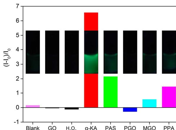
**Fig. 4** Fluorescence response of probe **3** upon various dicarbonyls and ROS. Probe **3** (10  $\mu\text{M}$ ) with CTAB (1 mM) was incubated with 100  $\mu\text{M}$  substrate for 10 min at 20  $^{\circ}\text{C}$  in PBS (pH 6.0). Substrates are glyoxal (GO), hydrogen peroxide ( $\text{H}_2\text{O}_2$ ),  $\alpha$ -ketoglutaric acid ( $\alpha$ -KA), sodium pyruvate (PAS), phenylglyoxal (PGO), methylglyoxal (MGO) and phenylpyruvic acid (PPA).
