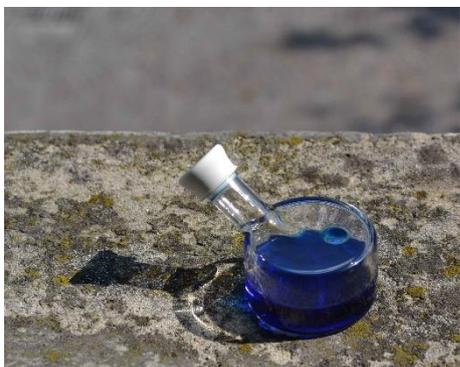
**Figure 1.** Pyrex glass vessel (20 mL capacity) used for the sunlight photocatalyzed  $\beta$ -C-H/C-C conversion of **1a**.
