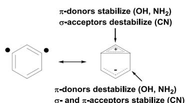
Fig. 3 Substituent effects on the stability of a bicyclic zwitterionic resonance structure of *meta*-benzynes.
