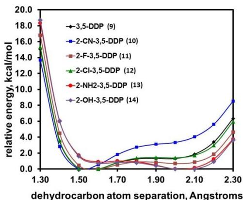
Fig. 7 Relative energy versus dehydrocarbon atom separation (DAS) for 9–14 (DDP = didehydropyridinium cation) calculated at the RHF–UCCSD(T)/cc–pVTZ//B3LYP/cc–pVTZ level of theory.
