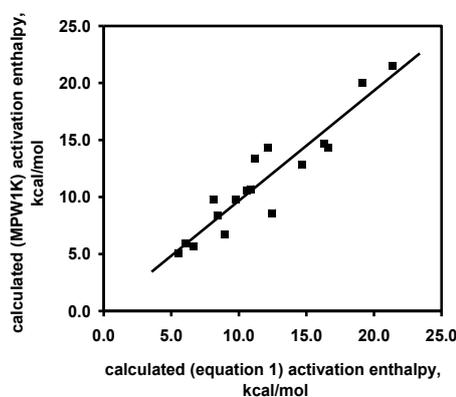
Fig. 9 Calculated (MPW1K) activation enthalpies versus calculated (equation 1) activation enthalpies for hydrogen atom abstraction from methane (as a model for cyclohexane) by biradicals **4–20**. The data are fit to a linear trend line ( $y = 0.9653x + 0.0205$ ;  $R^2 = 0.8799$ ).
