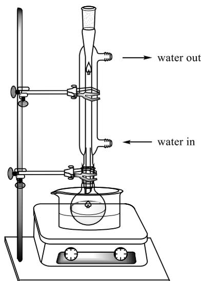
Figure A: The apparatus for the synthesis of tin (IV) iodide.
