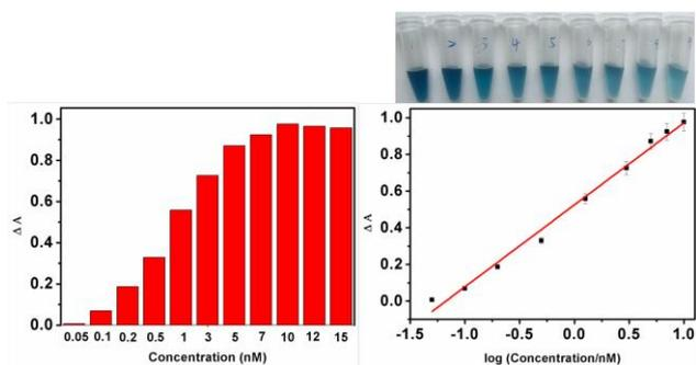
Fig. 3 (A)  $\Delta A$  at 650 nm in the presence of various concentration of ricin. (B) Typical calibration curve for ricin obtained using the colorimetric aptasensor. Inset shows the corresponding digital images.
