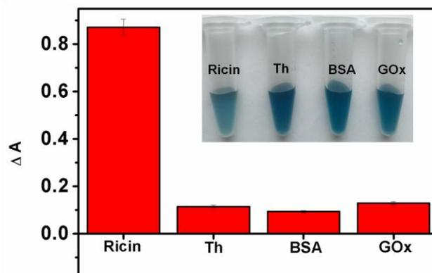
Fig. 4 The selectivity of the proposed system towards ricin detection. The concentration of ricin and other proteins are 7 nM. Inset shows the corresponding digital images.
