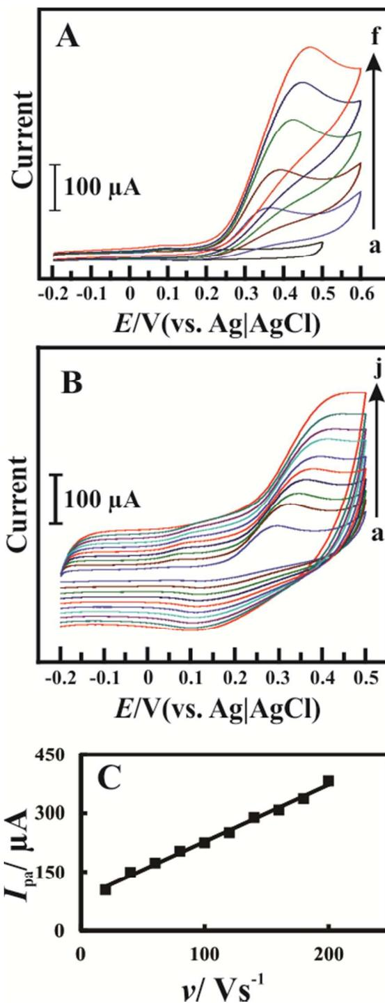
**Fig. 4** A) Cyclic voltammograms obtained at MWCNT-CoTsPc/GCE in the absence (a) and presence of each 1 mM glucose addition (b-f) in 0.1M NaOH at a scan rate  $50 \text{ mV s}^{-1}$ . B) The cyclic voltammetry response of MWCNT-CoTsPc/GCE in 0.1 NaOH containing 1 mM glucose at different scan rates from 0.01 to  $0.1 \text{ Vs}^{-1}$  (a to j). C) Linear plot for  $I_{pa}$  vs. scan rates.
