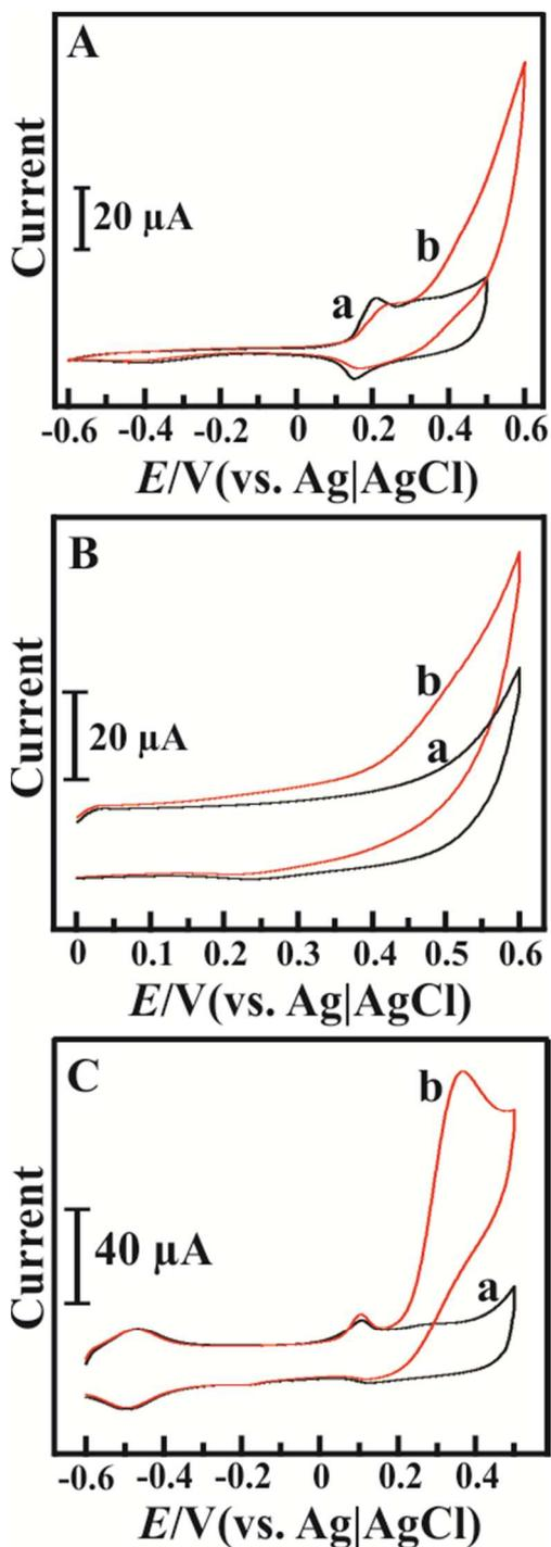
**Fig. 3** Cyclic voltammograms obtained at GCE electrode modified with CoTsPc (A), MWCNT (B) and MWCNT-CoTsPc (C) in the absence (a) and presence of 1 mM glucose (b) in 0.1M NaOH at a scan rate of  $50 \text{ mV s}^{-1}$ .
