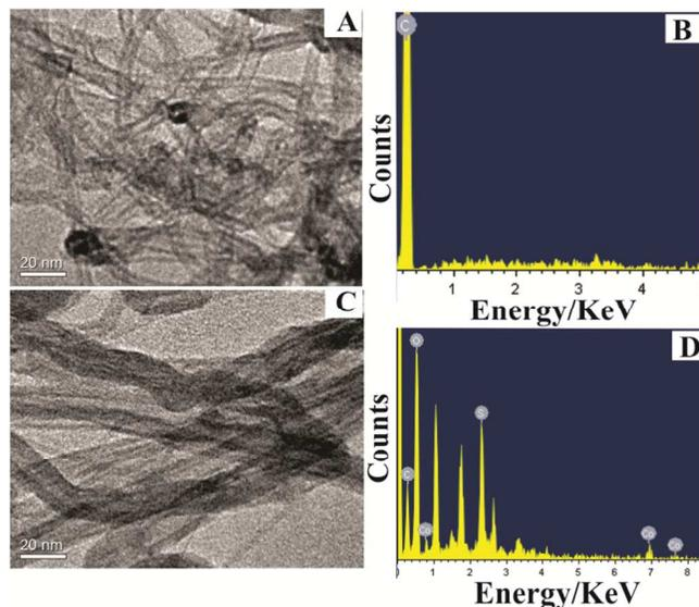
**Fig. 1** TEM image of pristine MWCNT (A) and MWCNT-CoTsPc (B). EDX spectra of MWCNT (C) and MWCNT-CoTsPc (D).
