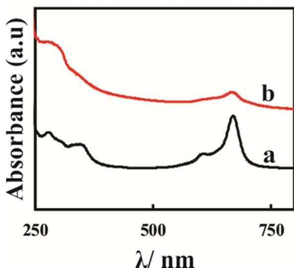
**Fig. 2** UV-Visible spectra of CoTsPc (a) and MWCNT-CoTsPc (b).
