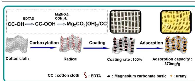
Sch. 1 Schematic diagram of preparation and adsorption.
