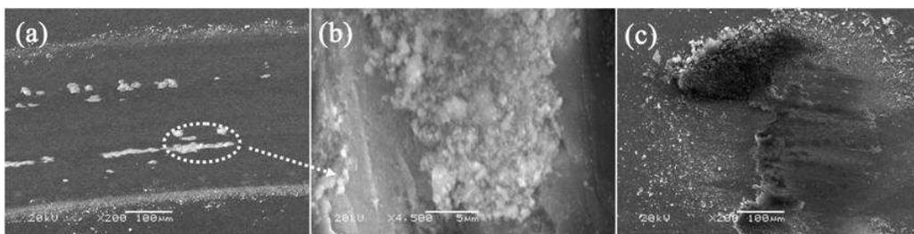
**Figure 5.** SEM images of worn surfaces of a-C:H film (a, b) and steel ball counterface (c) after 1000 cycles
