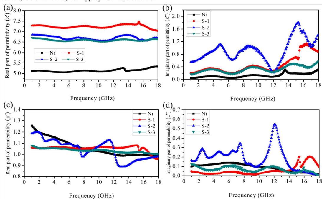
Fig. 6 Frequency dependence of the (a) real and (b) imaginary parts of complex permittivity, and the (c) real and (d) imaginary parts of complex permeability for the Ni and three Ni/ZnS samples.
