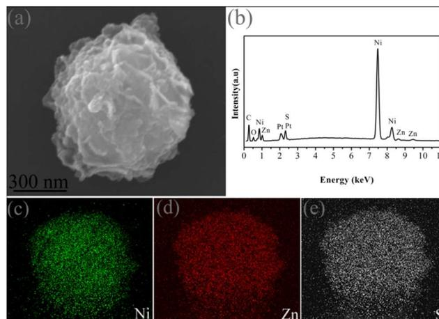
**Fig. 3** (a) FESEM image of an individual Ni/ZnS composites, (b) EDS pattern of Ni/ZnS composite and (c-e) corresponding elemental mappings of Ni, Zn and S.
