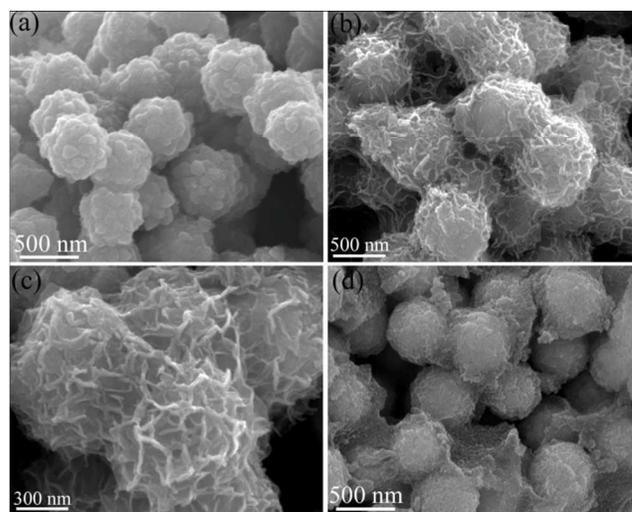
**Fig. 5** FESEM images of hierarchical Ni/ZnS core-shell composites prepared at different temperature: (a) S-1 (40 °C); (b, c) S-2 (60 °C); (d) S-3 (80 °C).
