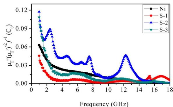
Fig. 9 The value  $C_0$  ( $\mu''(\mu')^{-2} f^{-1}$ ) of Ni particles and Ni/ZnS composite as a function of frequency.
