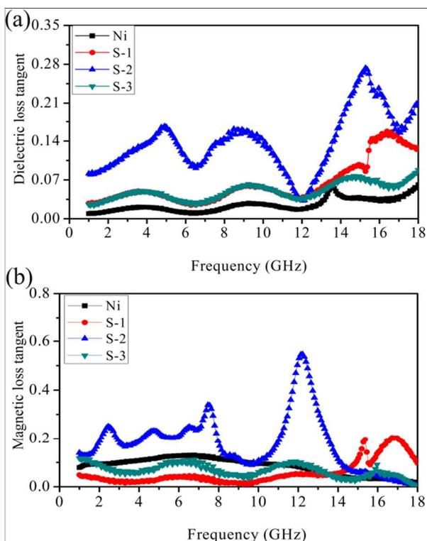
Fig. 7 (a) The dielectric loss factor and (b) magnetic loss factor of Ni particles and Ni/ZnS–paraffin wax samples versus frequency.
