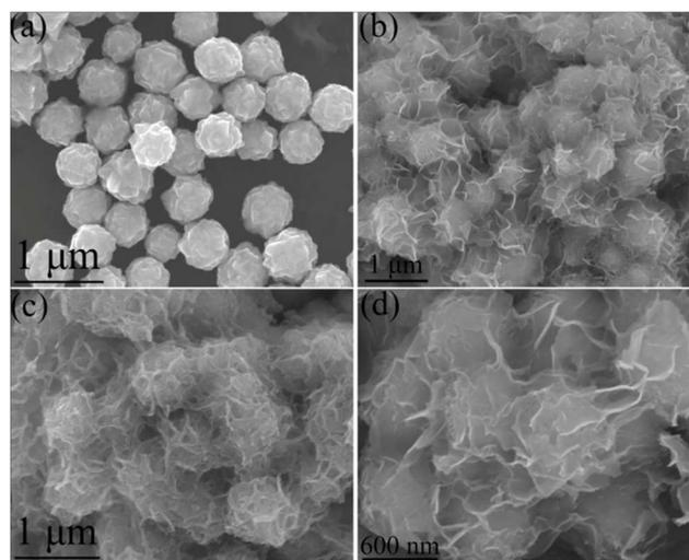
**Fig. 2** (a) FESEM image of Ni walnuts and (b-d) different magnification FESEM images of ZnS nanonet-wrapped Ni composites.
