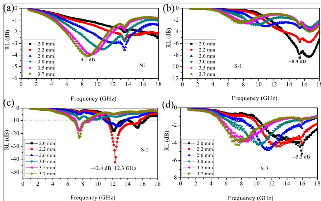
**Fig. 11** The reflection losses of (a) Ni particles, (b) S-1, (c) S-2 and (d) S-3 samples with various thicknesses.
