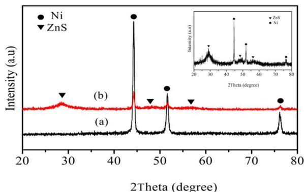
**Fig. 1** XRD patterns of (a) walnut-like Ni particle and (b) core-shell Ni/ZnS composites. Inset is the XRD profile of Ni/ZnS composite.
