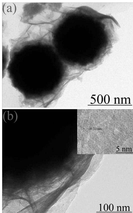
**Fig. 4** TEM images of crumpled ZnS net-wrapped Ni walnut sphere composite with different magnifications. Inset of (b) shows the HRTEM of ZnS shell.
