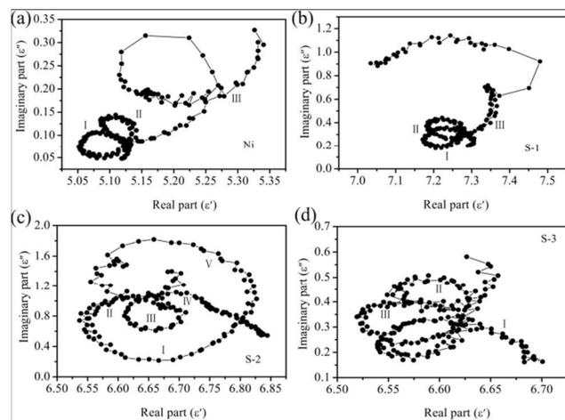
Fig. 8 Typical Cole-Cole semicircles ( $\epsilon''$  versus  $\epsilon'$ ) for Ni particles and Ni/ZnS composites in the frequency range of 1-18 GHz.
