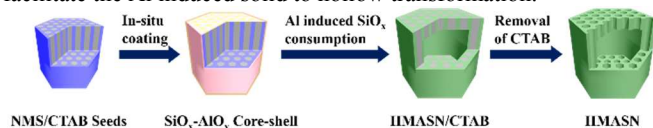
Scheme 1 Proposed formation mechanism of HMASN.
