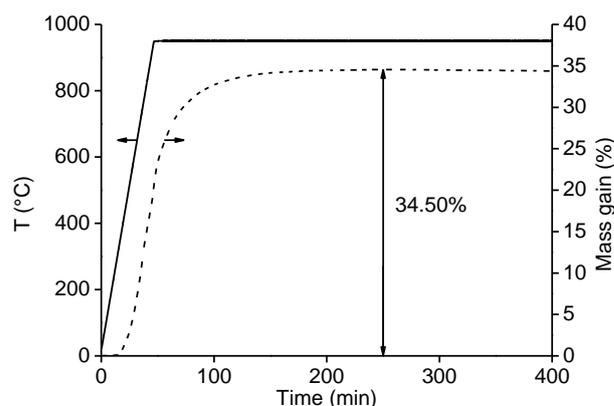
Fig. 2 Thermogravimetric analysis of the magnet powder  $<400\ \mu\text{m}$ . The NdFeB magnet powder was first heated to 950  $^{\circ}\text{C}$  (heating rate: 20  $^{\circ}\text{C}\ \text{min}^{-1}$ ) and kept at this temperature for another 6 h. The temperature of the furnace is given by the solid line and the mass gain (%) by the dashed line.
