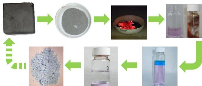
A recycling process was developed in which only oxalic acid is consumed to remove and separate the rare-earth metals from NdFeB magnets.
