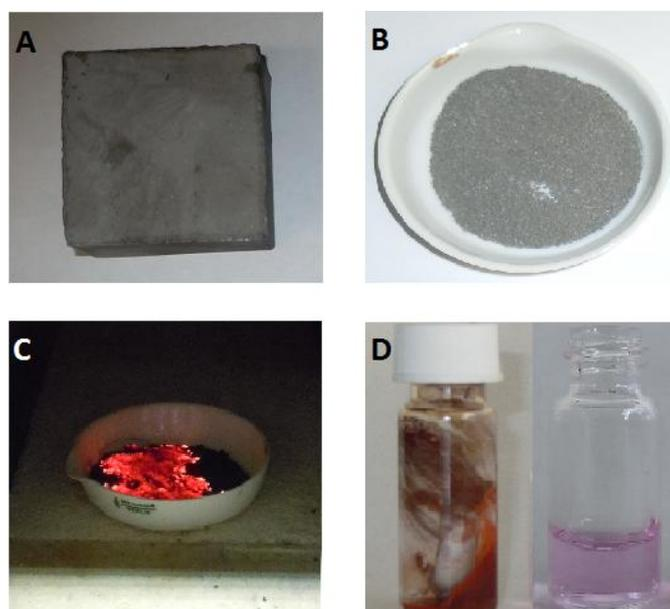
Fig. 1 (A) The NdFeB magnet before crushing and milling, (B) NdFeB powder (<400 µm) before roasting, (C) roasting and powder fire at high temperatures and (D) the leachate colored pink-violet by neodymium (right) and the remaining orange/brown iron(III) hydroxide precipitate (left).
