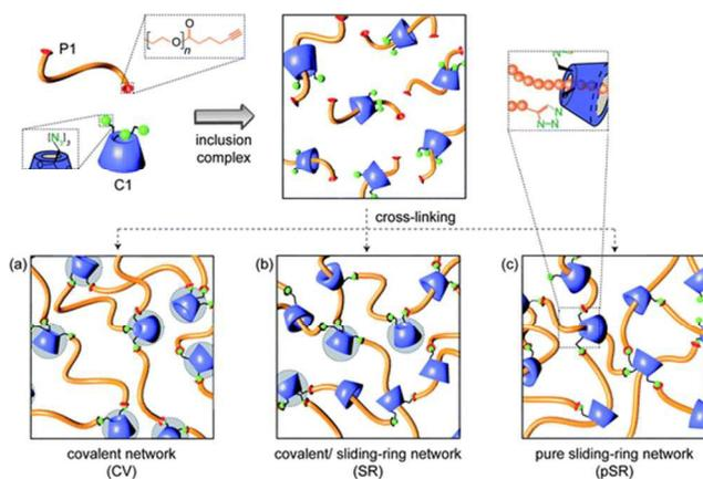
**Figure 1.** Schematic representation of the formation of  $\alpha$ -cyclodextrin ( $\alpha$ CD)-polyethylene glycol(PEG) hydrogels through the formation of alkyne-azide chemistry (CV), inclusion complexes (pSR) and a combination of both (SR). Reproduced from reference 95 with permission from RSC Publishing.
