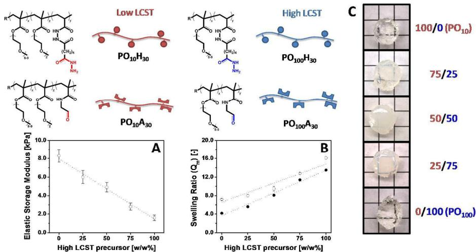
**Figure 7.** Tuning hydrogel properties by mixing POEGMA precursors of different LCST. (A) Elastic storage modulus ( $G'$ ), (B) mass-based swelling ratio ( $Q_m$ ) and (C) physical appearance of POEGMA hydrogels containing 100/0, 75/25, 50/50, 25/75 and 0/100 w/w% PO<sub>10</sub>H<sub>30</sub>/PO<sub>100</sub>H<sub>30</sub> and PO<sub>10</sub>A<sub>30</sub>/PO<sub>100</sub>A<sub>30</sub>. Data reproduced from references 155 and 157 with permission from Wiley-VCH and ACS.
