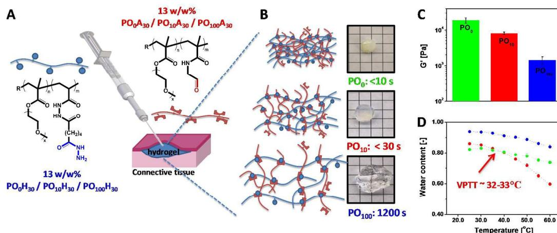
**Figure 6.** (A) Preparation of POEGMA hydrogels using a double-barrel syringe. (B) Physical appearance and gelation time for PO<sub>0</sub>, PO<sub>10</sub> and PO<sub>100</sub> hydrogels. (C) Hydrogel mechanics as measured by the shear storage modulus ( $G'$ ). (D) Thermoresponsive
