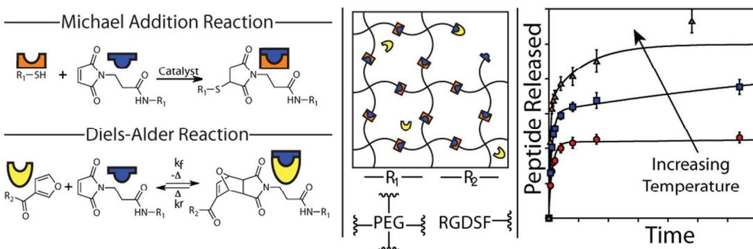
**Figure 3.** The formation of PEG hydrogels using thiol-Michael addition and the functionalization with a releasable fluorescent RGD peptide using Diels-Alder chemistry. A schematic representation of the hydrogel network and the release kinetics as a function of the temperature are also shown. Reproduced from reference 48 with permission from ACS publishing.
