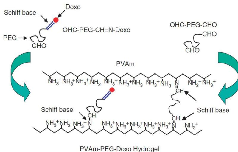
**Figure 4.** Schematic representation of the formation of poly(vinylamine) (PVAm)-poly(ethylene glycol) (PEG)-doxorubicin(doxo) hydrogels using Schiff base chemistry. Reproduced from reference 52 with permission from SAGE journals.
