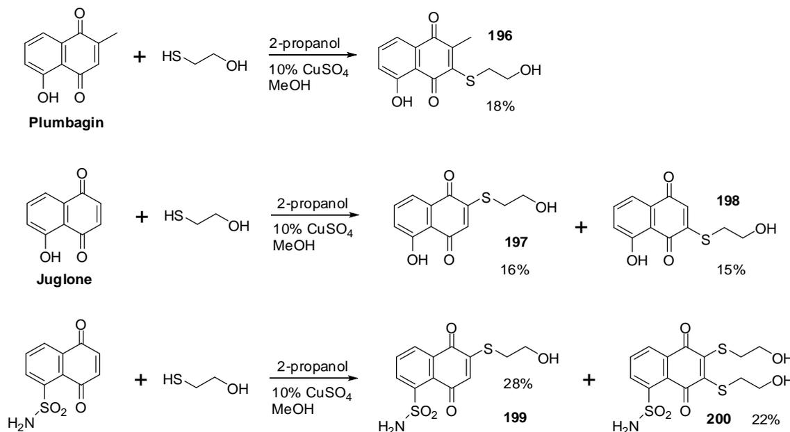
**Scheme 7.** Synthesis of mono- and dithiolated naphthoquinone derivatives **196-200**.
