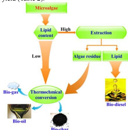
Fig. 4 Possible microalgal processing options based on lipid content
