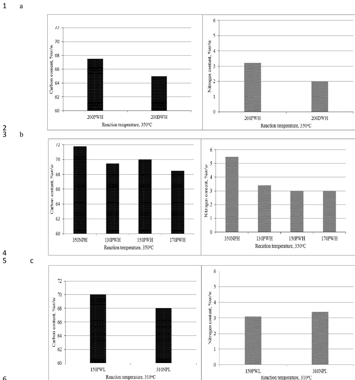
Figure 6: Elemental composition of biocrude from pretreated and untreated algae at different reaction condition.
