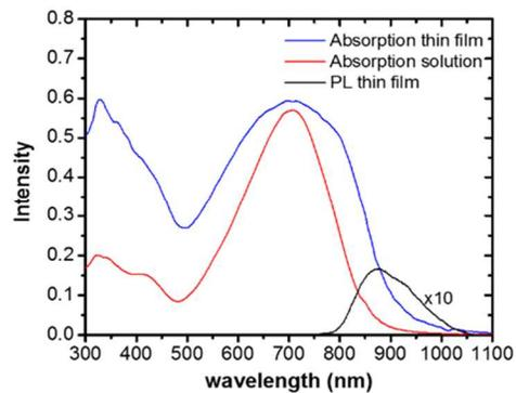
**Fig. 2** Absorption spectra of TDPPTTB in chloroform solution and as thin film
