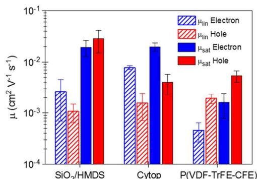
**Fig. 7** Mobilities ( $\mu$ ) of TDPPTB transistors based on different dielectrics. All values are calculated from  $120 \text{ }^\circ\text{C}$ -annealed TDPPTB films.
