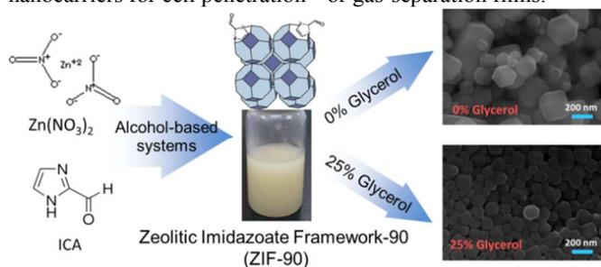
**Scheme 1.** Synthesis of ZIF-90 nanoparticles with ~100 nm particle size prepared by changing the viscosity using glycerol in a water-alcohol-based system
