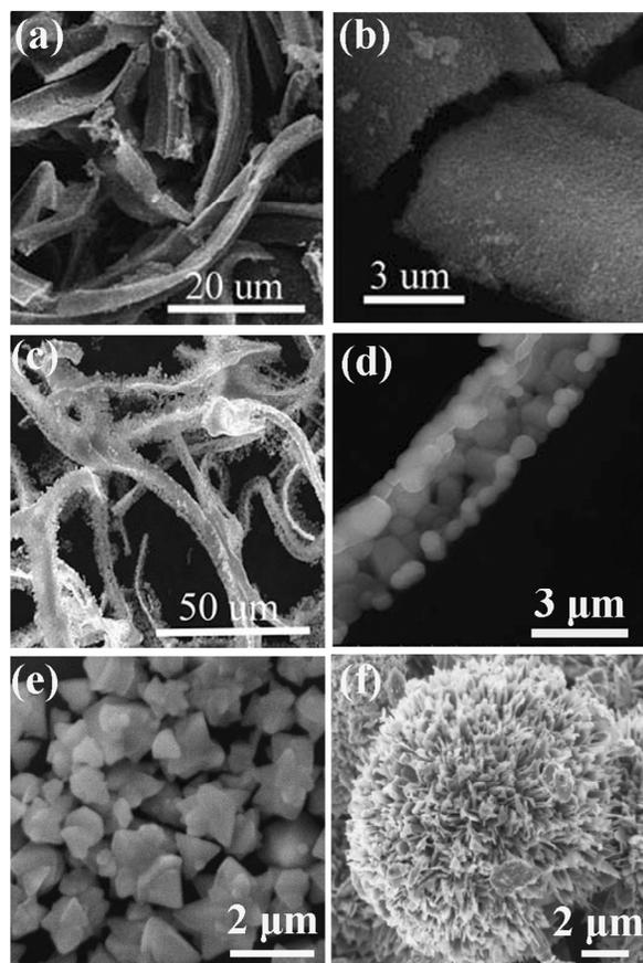
**Fig. 5** SEM images of the ZnO post-annealing at 600 °C (a, b),<sup>85</sup> SrAl<sub>x</sub>O<sub>y</sub> post-annealing at 1300 °C (c, d),<sup>86</sup> triangular ZnO (e),<sup>87</sup> and CuO nanoflowers (f).<sup>88</sup> (e) adopted from Ref. 87, Copyright 2009, with permission from American Chemical Society. (f) adopted from Ref. 88, Copyright 2013, with permission from Elsevier.
