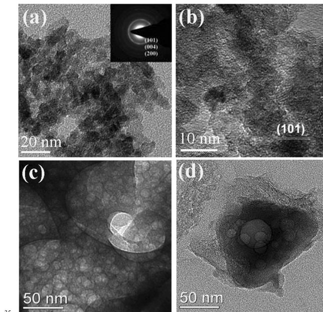
**Fig. 6** (a) TEM image and (b) HRTEM image of TiO<sub>2</sub> with wormhole mesopores.<sup>98</sup> (c, d) TEM images of porous Li<sub>3</sub>V<sub>2</sub>(PO<sub>4</sub>)<sub>3</sub>/C.<sup>61</sup> (c), (d) adopted from Ref. 61, Copyright 2012, with permission from Elsevier.
