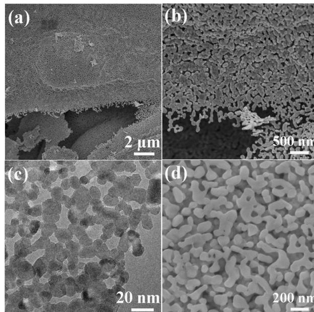
**Fig.8** (a, b) SEM images of porous ZnO network.<sup>110</sup> (c) TEM image of mesoporous  $\text{Co}_3\text{O}_4$  calcined at 355 °C.<sup>111</sup> (d) SEM image of macroporous
