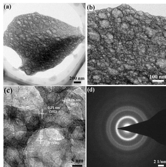
**Fig. 10** TEM images (a, b), HRTEM image (c), and (d) of porous ZnO nanofoams derived from focused electron beam irradiation of the zinc hydrazine complex under TEM operation.
