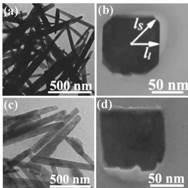
**Fig. 4** TEM images of (a, b)  $\text{Al}_4\text{B}_2\text{O}_9$  nanowires synthesized at 900 °C for 2 h and (c, d)  $\text{Al}_{18}\text{B}_4\text{O}_{33}$  Nanowires synthesized at 1050 °C for 2 h.<sup>84</sup> Adopted from Ref. 84, Copyright 2007, with permission from American Chemical Society.
