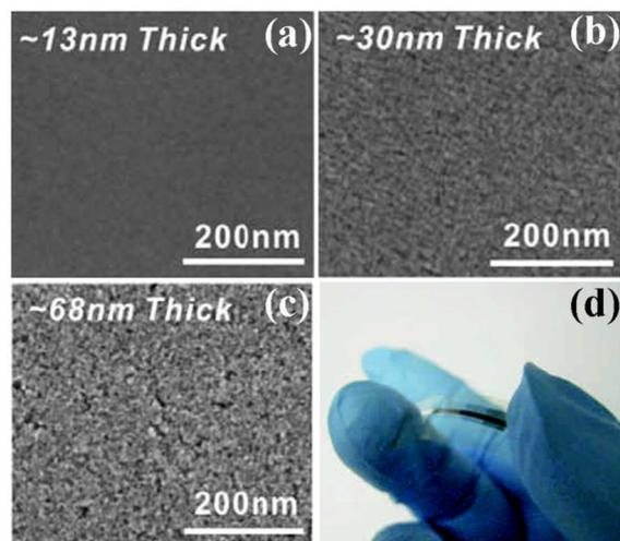
**Fig. 11** (a-c) SEM images of In<sub>2</sub>O<sub>3</sub> films on n++ Si with controlled thickness. (d) Optical image of a flexible combustion-processed In<sub>2</sub>O<sub>3</sub> device.<sup>51</sup> Adopted from Ref. 51, Copyright 2011, with permission from Macmillan Publishers Ltd.
