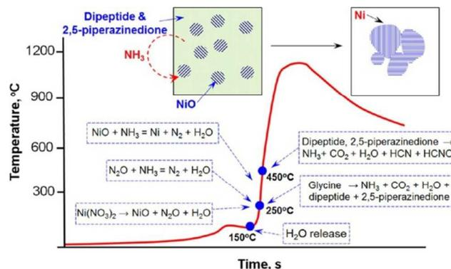
Fig. 2 A schematic illustration showing the mechanism of Ni formation during self-sustained combustion reactions of nickel nitrate-glycine gels.<sup>74</sup> Adopted from Ref. 74, Copyright 2013, with permission from American Chemical Society.
