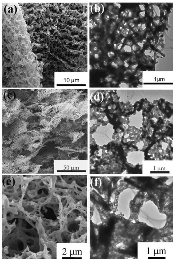
**Fig. 9** SEM image (a) and TEM image (b) of 3D macroporous NiO/Ni. SEM image (c) and TEM image (d) of 2D macroporous NiO/Ni.<sup>115</sup> SEM image (e) and TEM image (f) of 3D porous ZnO.<sup>116</sup> (a)-(d) adopted from Ref. 115, Copyright 2013, with permission from Elsevier.
