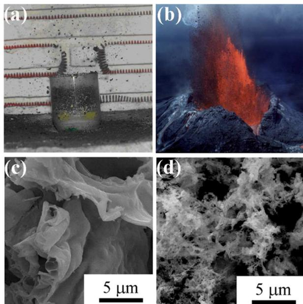
15 **Fig. 7** Optical photographs of eruption combustion process (a) and volcanic eruption in nature (b). The optical photograph showing a natural volcanic eruption is from the Internet. SEM images of Ni/NiO powders derived with conventional combustion (c) and eruption combustion (d).<sup>108</sup> Adopted from Ref. 108, Copyright 2011, with permission from American
