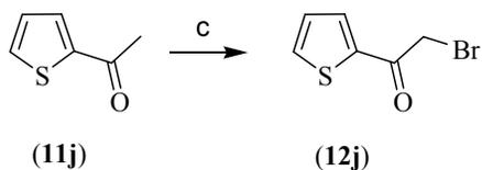
Reagents and conditions: (a) Bromine, diethyl ether, DCM, 0 °C to rt, 2h; (b) Bromine, 33% HBr in acetic acid, 0 to 60 °C, 2h; (c) Bromine, DCM, rt, 2h.
