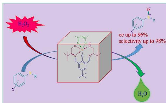
This study represents the rare combination of non-toxic Fe based catalyst/H<sub>2</sub>O<sub>2</sub> as an efficient catalytic protocol for asymmetric sulfoxidation reaction.
