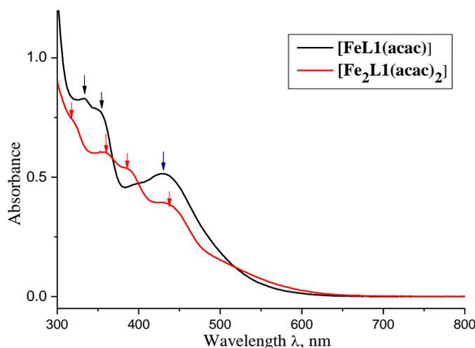
**Fig. 1** UV vis. spectra of *in situ* generated complex with metal to ligand ratio of 1:1 and 2:1.
