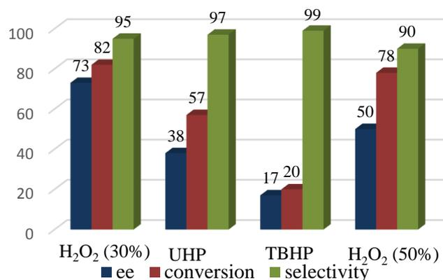
**Fig. 2** Effect of oxidant on the enantioselective oxidation of methyl phenyl sulfide, catalyzed by *in situ* generated  $[\text{FeL1}(\text{acac})]$  complex in  $\text{CH}_2\text{Cl}_2$  at RT.
