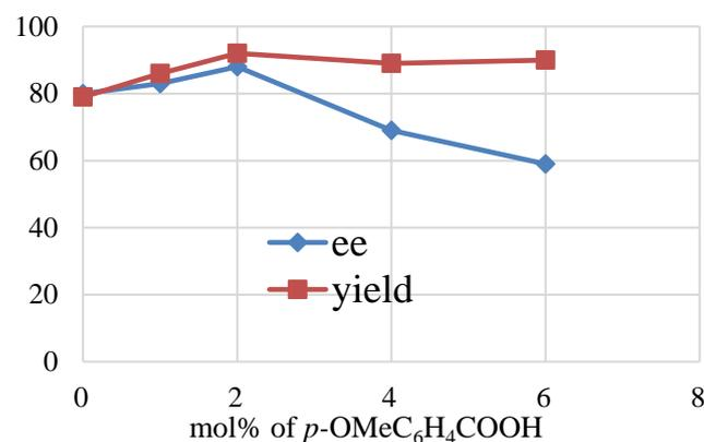
**Fig. 3** Effect of the concentration of *p*-OMeC<sub>6</sub>H<sub>4</sub>COOH as additive on enantioselective oxidation of methyl phenyl sulfide catalyzed by *in situ* generated [Fe**L1**(acac)] complex at 15 °C.
