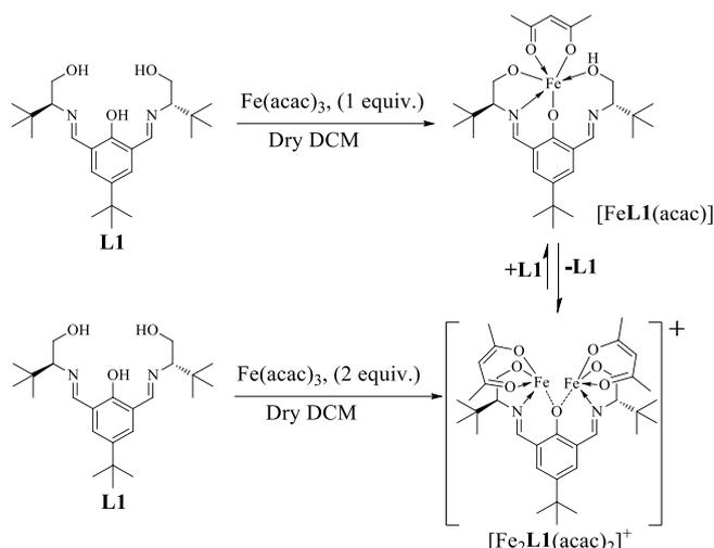
**Scheme 2** Plausible structures of the *in situ* generated monomeric  $[\text{FeL1}(\text{acac})]$  and dimeric  $[\text{Fe}_2\text{L1}(\text{acac})_2]^+$  complex.
