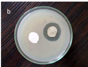
Figure 9(b)) Antibacterial activity of T-PEUU fiber mat ( $\sim 0.7$  mg) and PEUU mat against *Escherichia coli* 14x10mm (300 x 300 DPI)
