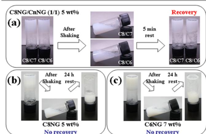
**Fig. 1** Images of hydrogels before, during and after gelation and thixotropic tests. (a) C8NG/CnNG 1/1 (w/w) 5 wt%, (b) C8NG 5 wt%, and (c) C6NG 7 wt% hydrogels.
