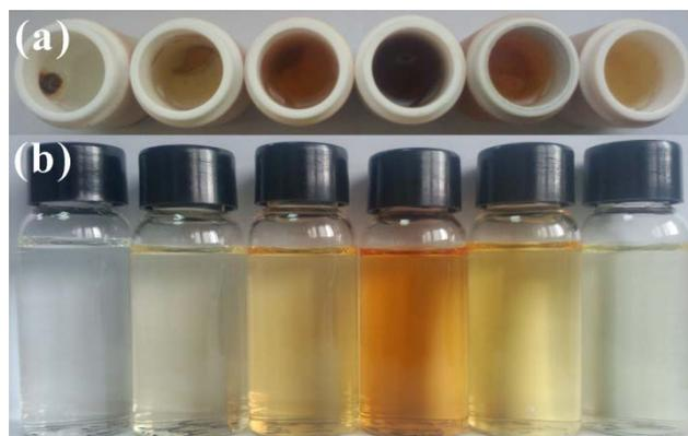
**Fig. 1** (a) The products of WPBs which were heated in different concentrations of H<sub>2</sub>O<sub>2</sub> (from left to right: 0.0, 0.2, 1.0, 2.0, 3.0, and 5.0 wt%) at 180 °C for 12 h, and (b) the centrifuged solutions of CNPs.
