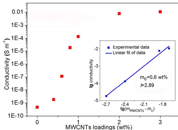
**Figure 6.** Dependence of the conductivity of PEEK/TPI/MWCNTs composites on the MWCNTs
