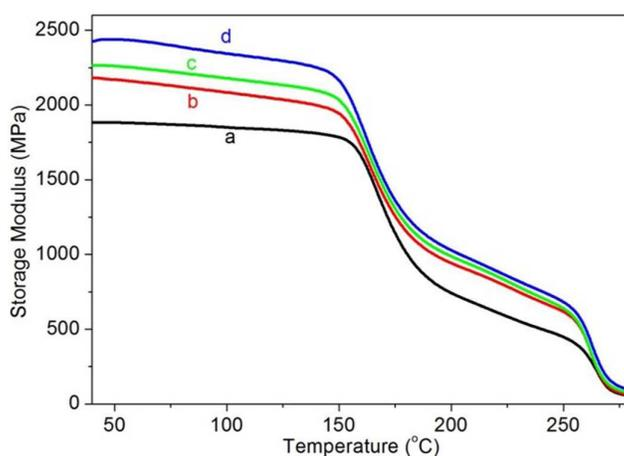
**Figure 8.** Storage modulus curves of (a) P/T, (b) P/T/0.4%-CNTs, (c) P/T/1%-CNTs and (d) P/T/3%-CNTs.
