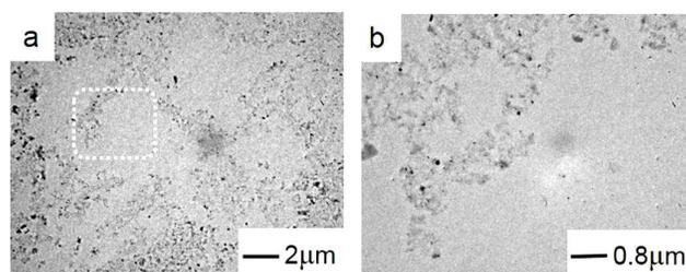
**Figure 3.** TEM images of (a) P/T/1%-CNTs, (b) magnified micrograph of the dotted-line circle region.
