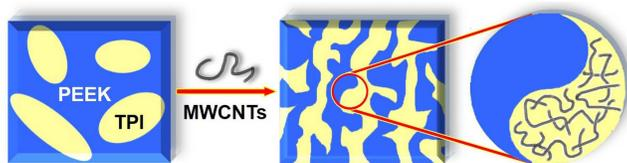
**Figure 5.** Schematic representation of MWCNTs induced co-continuity of PEEK/TPI blend.
