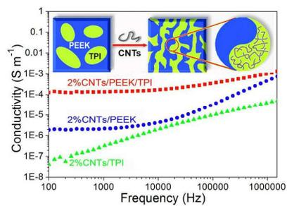
High performance conductive material was prepared based on MWCNTs induced co-continuity of PEEK/TPI blends.
