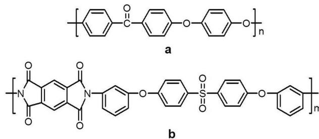
**Figure 1.** Structure of (a) PEEK and (b) TPI.
