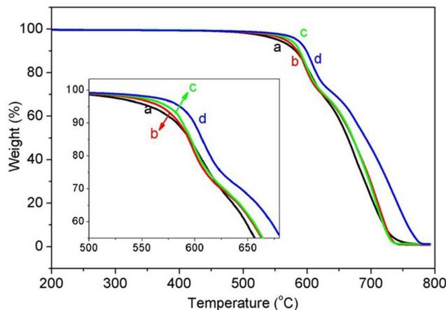
**Figure 9.** TGA curves of (a) P/T, (b) P/T/0.4%-CNTs, (c) P/T/1%-CNTs and (d) P/T/3%-CNTs.
