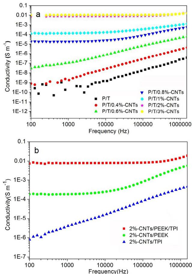
**Figure 7.** (a) Dependence of AC conductivity of PEEK/TPI/MWCNTs composites with different MWCNTs content on frequency. (b) Dependence of AC conductivity of different polymer-based composites with 2 wt% MWCNTs on frequency.
