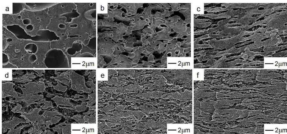
**Figure 4.** SEM images of PEEK/TPI composites with different contents of MWCNTs. (a) P/T, (b) P/T/0.4%-CNTs, (c) P/T/0.8%-CNTs, (d) P/T/1%-CNTs, (e) P/T/2%-CNTs, (f) P/T/3%-CNTs.
