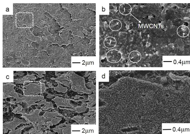
**Figure 2.** SEM images of (a) un-etched fractured surface of P/T/1%-CNTs, (b) magnified micrograph of the dotted-line circle region of (a), (c) etched fractured surface of P/T/1%-CNTs, (d) magnified micrograph of the dotted-line circle region of (c).
