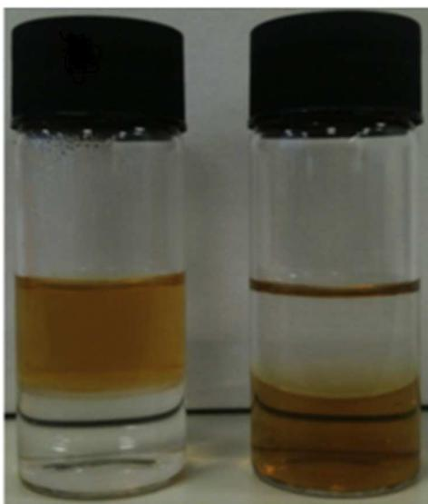
**Fig. 45.** Photographs of  $\text{MnFe}_2\text{O}_4$  (left) and  $\text{MnFe}_2\text{O}_4@\text{Al}(\text{OH})_3$  (right) NPs in a two-phase mixture of hexane (upper layer) and water (lower layer).
