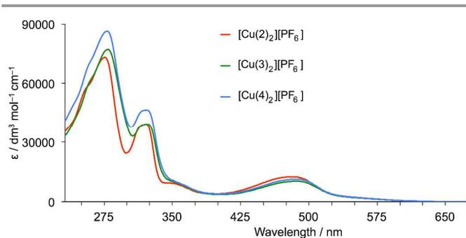
Fig. 6. Solution ( $\text{CH}_2\text{Cl}_2$ ) absorption spectra of the fluoro, chloro and bromo-containing complexes  $[\text{Cu}(\mathbf{2})_2][\text{PF}_6]$ ,  $[\text{Cu}(\mathbf{3})_2][\text{PF}_6]$  and  $[\text{Cu}(\mathbf{4})_2][\text{PF}_6]$ .
