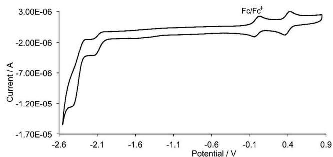
Fig. 7. Cyclic voltammogram for a  $\text{CH}_2\text{Cl}_2$  solution of  $[\text{Cu}(\mathbf{2})_2][\text{PF}_6]$ ; scan rate  $0.1 \text{ V s}^{-1}$  and referenced internally to  $\text{Fc}/\text{Fc}^+$ .
