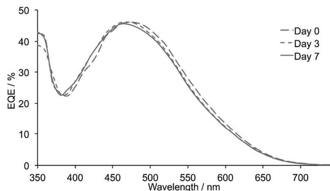
Fig. 12 EQE spectra measured over a 7 day period for one of the DSCs containing  $[\text{Cu}(\text{I})(\mathbf{5})]^+$  formed in situ by stepwise assembly.
