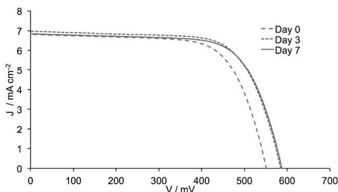
Fig. 11 J-V curves measured over a 7 day period for one of the DSCs containing  $[\text{Cu}(\text{I})(\mathbf{5})]^+$  formed in situ by stepwise assembly.
