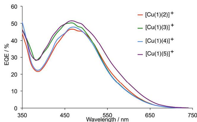
Fig. 10. Comparison of the EQE spectra for DSCs containing dyes  $[\text{Cu}(\mathbf{1})(\mathbf{2})]^+$  (fluoro),  $[\text{Cu}(\mathbf{1})(\mathbf{3})]^+$  (chloro),  $[\text{Cu}(\mathbf{1})(\mathbf{4})]^+$  (bromo) and  $[\text{Cu}(\mathbf{1})(\mathbf{5})]^+$  (iodo) measured 3 days after sealing the cells.
