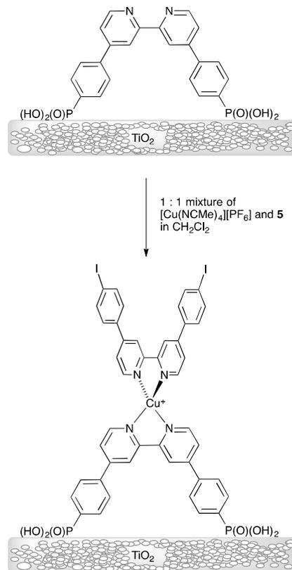
Scheme 4. Stepwise assembly of titania-anchored  $[\text{Cu}(\mathbf{1})(\mathbf{5})]^+$ .
