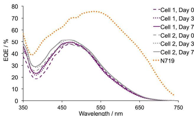
Fig. 9. EQE spectra for duplicate DSCs functionalized with  $[\text{Cu}(\mathbf{1})(\mathbf{5})]^+$  measured on the day of sealing the cell (day 0) and 3 and 7 days later, compared to the EQE spectrum of a DSC with N719.
