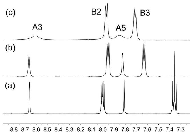
Fig. 2 500 MHz <sup>1</sup>H NMR spectra (aromatic region only) of CD<sub>3</sub>CN solutions of (a)  $[\text{Cu}(\mathbf{2})_2][\text{PF}_6]$ , (b)  $[\text{Cu}(\mathbf{3})_2][\text{PF}_6]$  and (c)  $[\text{Cu}(\mathbf{5})_2][\text{PF}_6]$  (see text).
