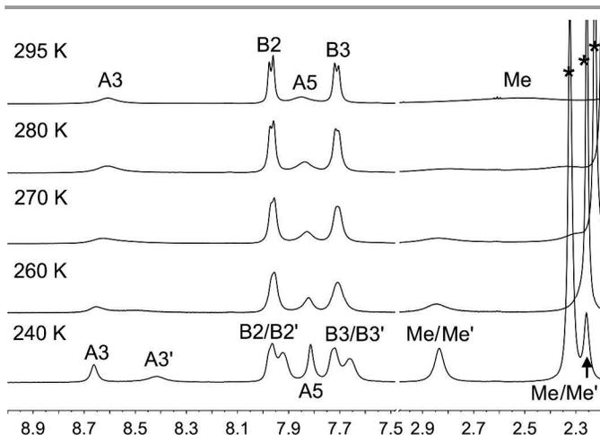
Fig. 3. Variable temperature 500 MHz  $^1\text{H}$  NMR spectra of the bulk material containing  $[\text{Cu}(\mathbf{5})_2][\text{PF}_6]$  and  $[\text{Cu}(\mathbf{5})(\text{MeCN})_2][\text{PF}_6]$ . \* = residual  $\text{H}_2\text{O}$  in  $\text{CD}_3\text{CN}$ .
