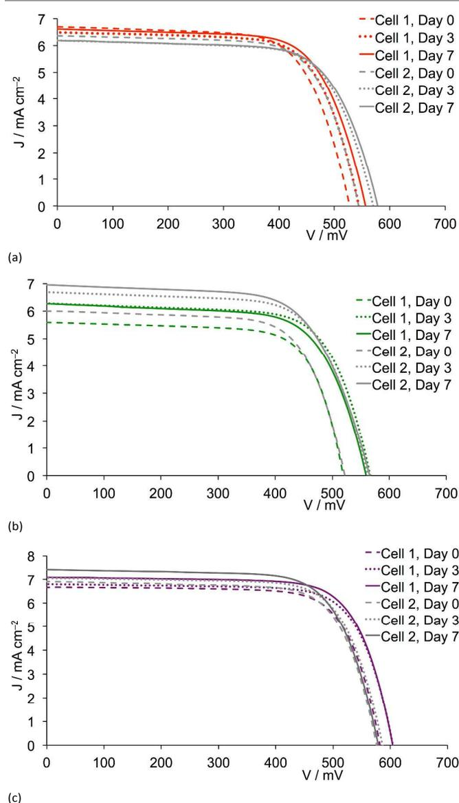
Fig. 8.  $J$ - $V$  curves for two independent DSCs containing dye (a)  $[\text{Cu}(\mathbf{1})(\mathbf{2})]^+$  (fluoro substituents), (b)  $[\text{Cu}(\mathbf{1})(\mathbf{3})]^+$  (chloro substituents) and (c)  $[\text{Cu}(\mathbf{1})(\mathbf{5})]^+$  (iodo substituents) measured over a 7 day period after sealing the cells.
