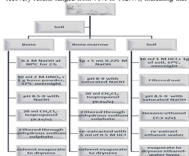
Scheme: 1 Flow chart of Extraction and sample preparation of bone, bone marrow and soil for codeine Sulphate
