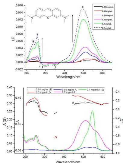
**Figure 4** (a) LD spectra of pyronin Y on PE<sup>OX</sup> deposited from solutions of concentrations indicated in the Figure. // and ⊥ indicate transition polarization with respect to the xantheno long axis in Figure 2. (b) Absorbance and LD<sup>r</sup> spectra of samples with concentrations 0.01 and 0.2 mg/ml overlaid with solution absorbance spectrum (S) and the dimer/monomer difference spectrum.
