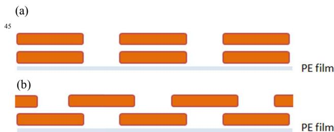
**Figure 8** (a) H-aggregate geometry which is consistent with the data for MeOH<sub>3</sub>-fluorone and pyronin Y at high concentrations. (b) Offset stacked geometry which is consistent with the data for pyronin B, fluorescein, and rhodamine 6G at high concentrations.
