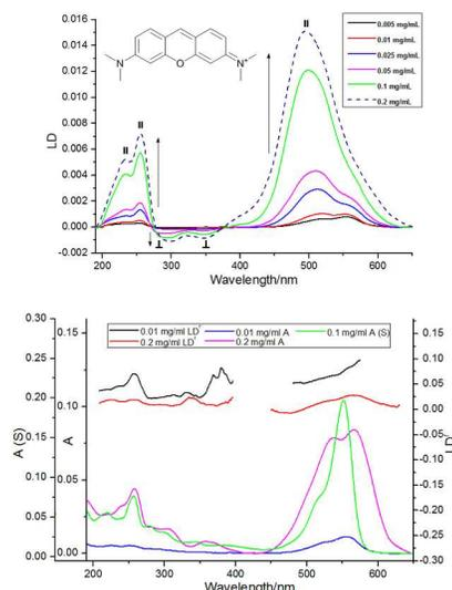
**Figure 5** (a) LD spectra of pyronin B on PEOX deposited from solutions of concentrations indicated in the Figure. // and ⊥ indicate transition polarization with respect to the xantheno long axis in Figure 2. (b) Absorbance and LD<sup>r</sup> spectra of samples with concentrations 0.01 and 0.2 mg/ml overlaid with solution absorbance spectrum (S) and the dimer/monomer difference spectrum.
