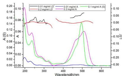
**Figure 6** (a) LD spectra of fluorescein on PE<sup>OX</sup> deposited from solutions of concentrations indicated in the Figure. // and  $\perp$  indicate transition polarization with respect to the xanthene long axis in Figure 2. (b) Absorbance and LD<sup>f</sup> spectra of samples with concentrations 0.01 and 0.2 mg/ml overlaid with solution absorbance spectrum (S) and the dimer/monomer difference spectrum.
