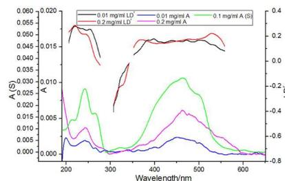
**Figure 3** (a) LD spectra of 9-methyl-2,3,7-trihydroxy-6-fluorone on PE<sup>OX</sup> deposited from 0.01 and 0.2 mg/mL solution and stretched by a factor of  $\times 2.4$ .  $\parallel$  and  $\perp$  indicate transition polarization with respect to the xanthene long axis in Figure 2. (b) Absorbance and LD<sup>f</sup> spectra of the LD spectra in Figure 3(a) overlaid with solution absorbance spectrum (denoted S).
