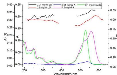
**Figure 7** (a) LD spectra of rhodamine 6G on PE<sup>OX</sup> deposited from solutions of concentrations indicated in the Figure. // and  $\perp$  indicate transition polarization with respect to the xanthene long axis in Figure 2. (b) Absorbance and LD<sup>f</sup> spectra of samples with concentrations 0.01 and 0.2 mg/ml overlaid with solution absorbance spectrum (S) and the dimer/monomer difference spectrum.
